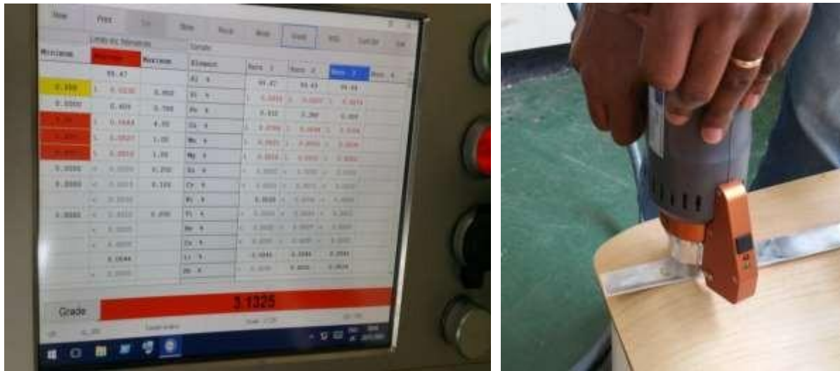
Figure 3.1. Chemical Compositions of aluminum alloy AA 2017
