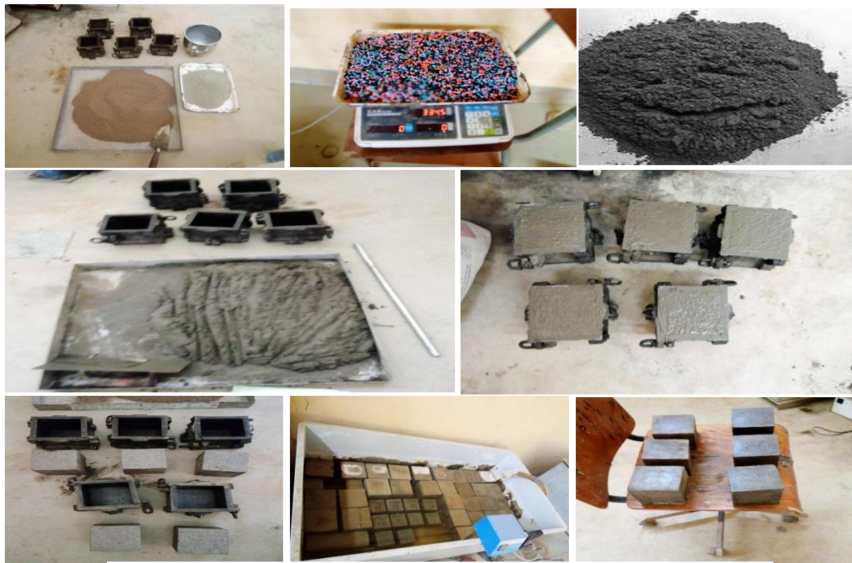
Figure 3. 5 cube test for mortar mixes
