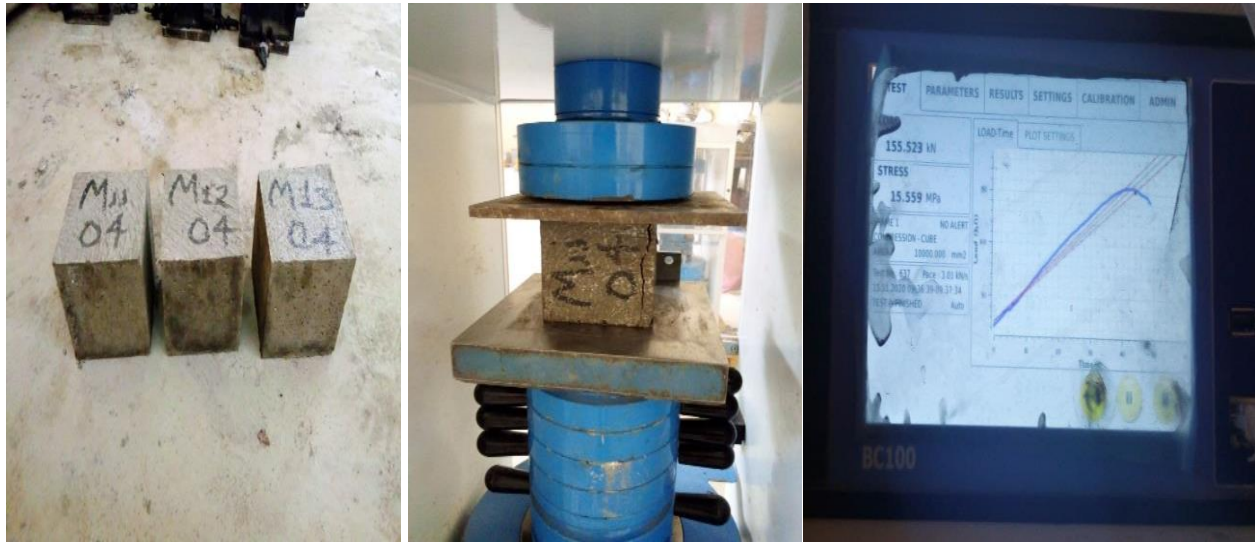
Figure 3. 10 compressive strength test and its output
