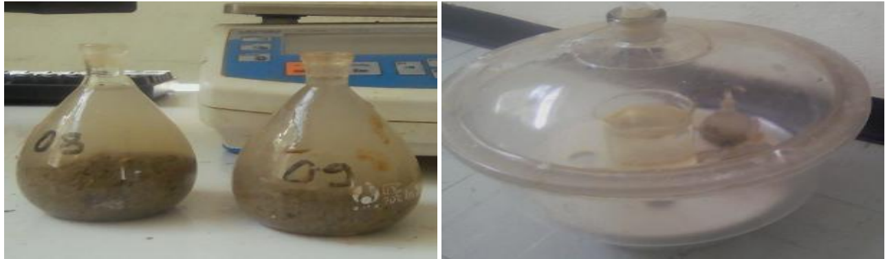
Figure 3.7: Specific gravity test (Taken on, 25/01/2021)
