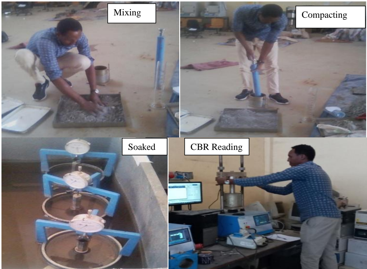
Figure 3.11: California bearing ratio test and procedures (Taken on, 15/03/2021)
