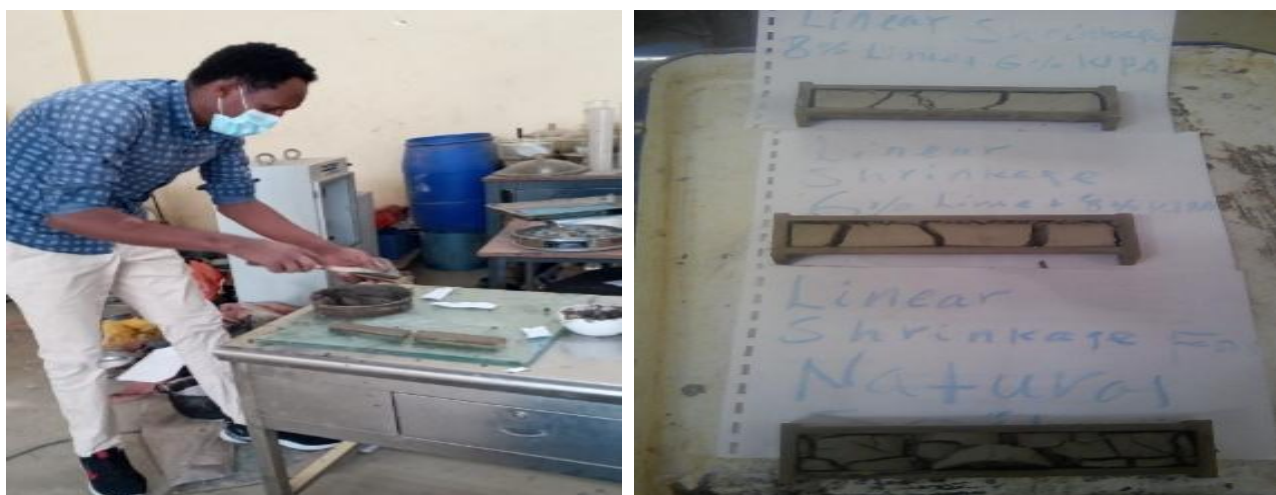
Figure 3.10: Linear shrinkage test (Taken on, 06/02/2021)
