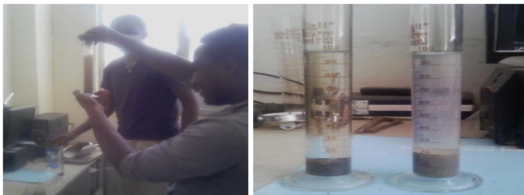
Figure 3.12: Free swell index test (Taken on, 27/01/2021)
