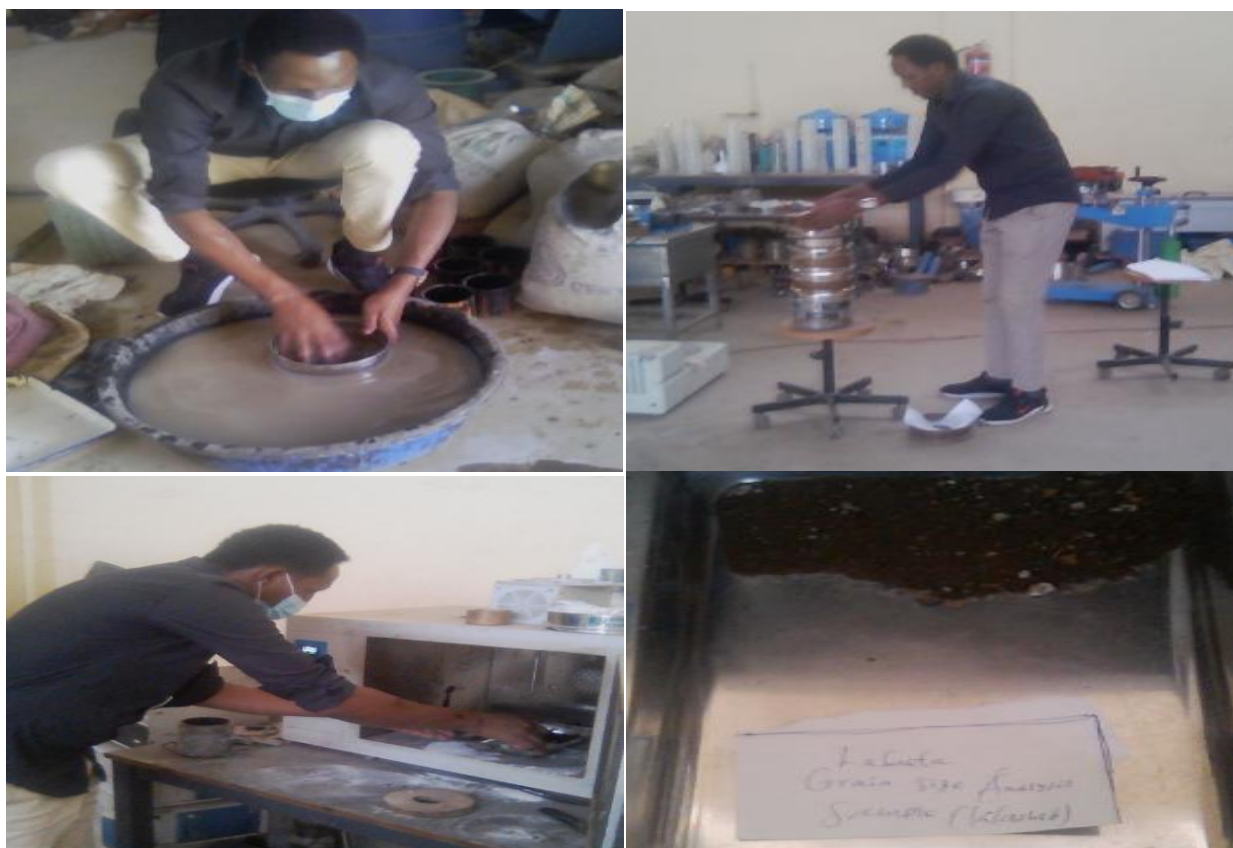
Figure 3.5: Wet sieve analysis procedures (Taken on, 27/01/2021)
