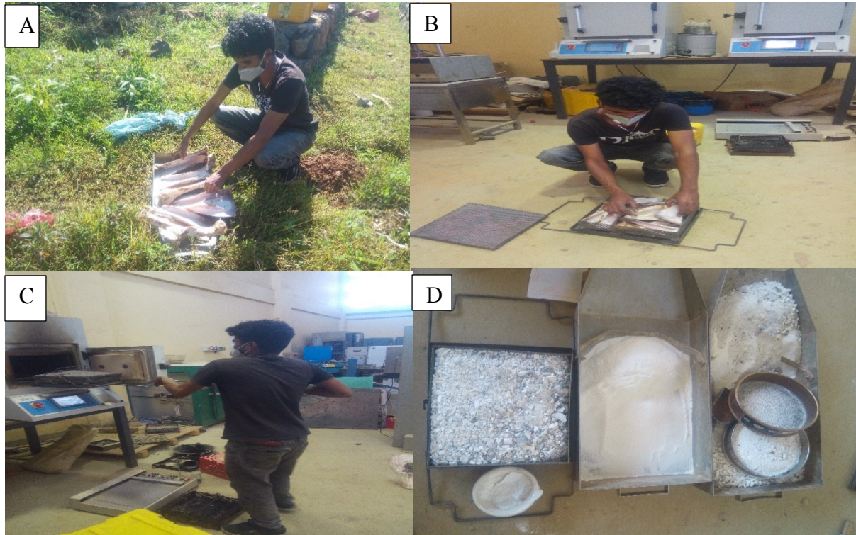
Figure 3.5: Preparation of bone ash (picture taken on 24/08/2020)
