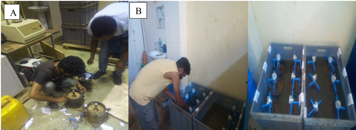
Figure 3.11: CBR test procedures (picture taken on 16/09/2020)
