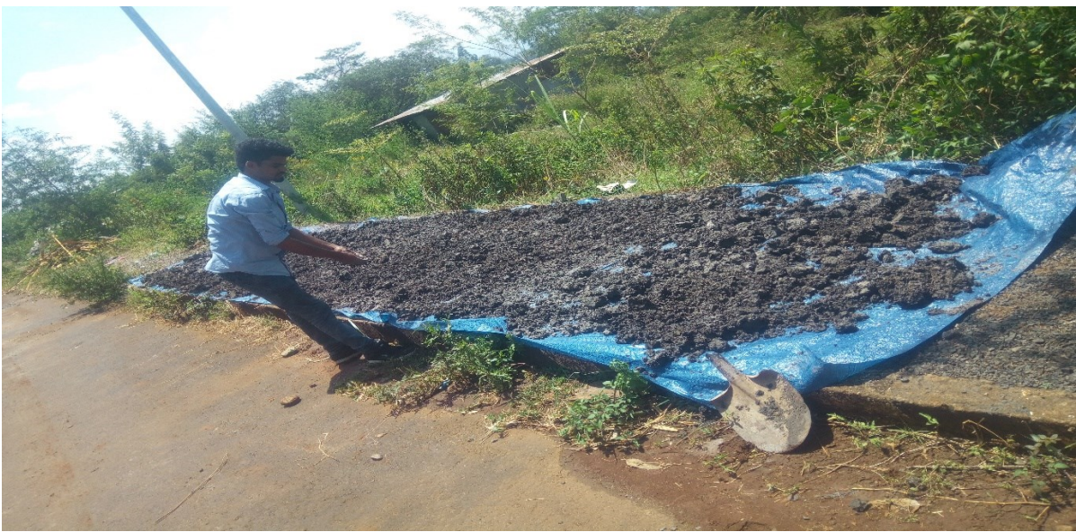
Figure 3.3: Black cotton soil sample preparation (picture taken on 21/08/2020)
