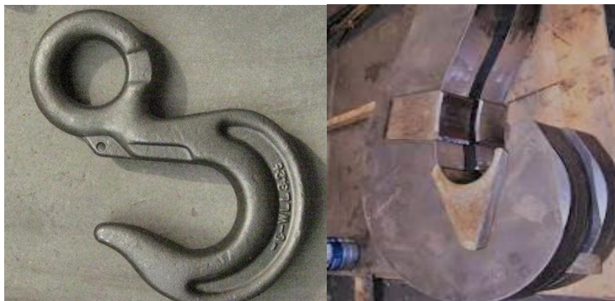
Figure 2. 3 a) forging crane hook, b) Laminated Crane Hook (Elebia.com, 2019)
