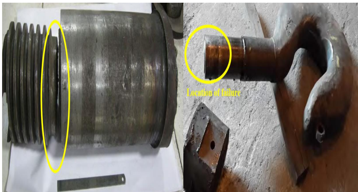
Figure 1.1 Overall view failure location of failed crane hook(Mukhopadhyay & Souvik, 2018).
