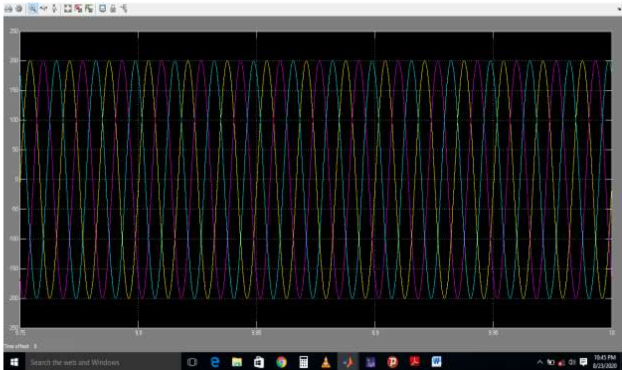
Figure 4.4 Oscillatory transient currents waveform with pre-insertion resistor.
