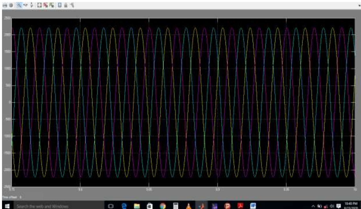
Figure 4.5 Oscillatory transient voltages waveform with pre-insertion inductor
