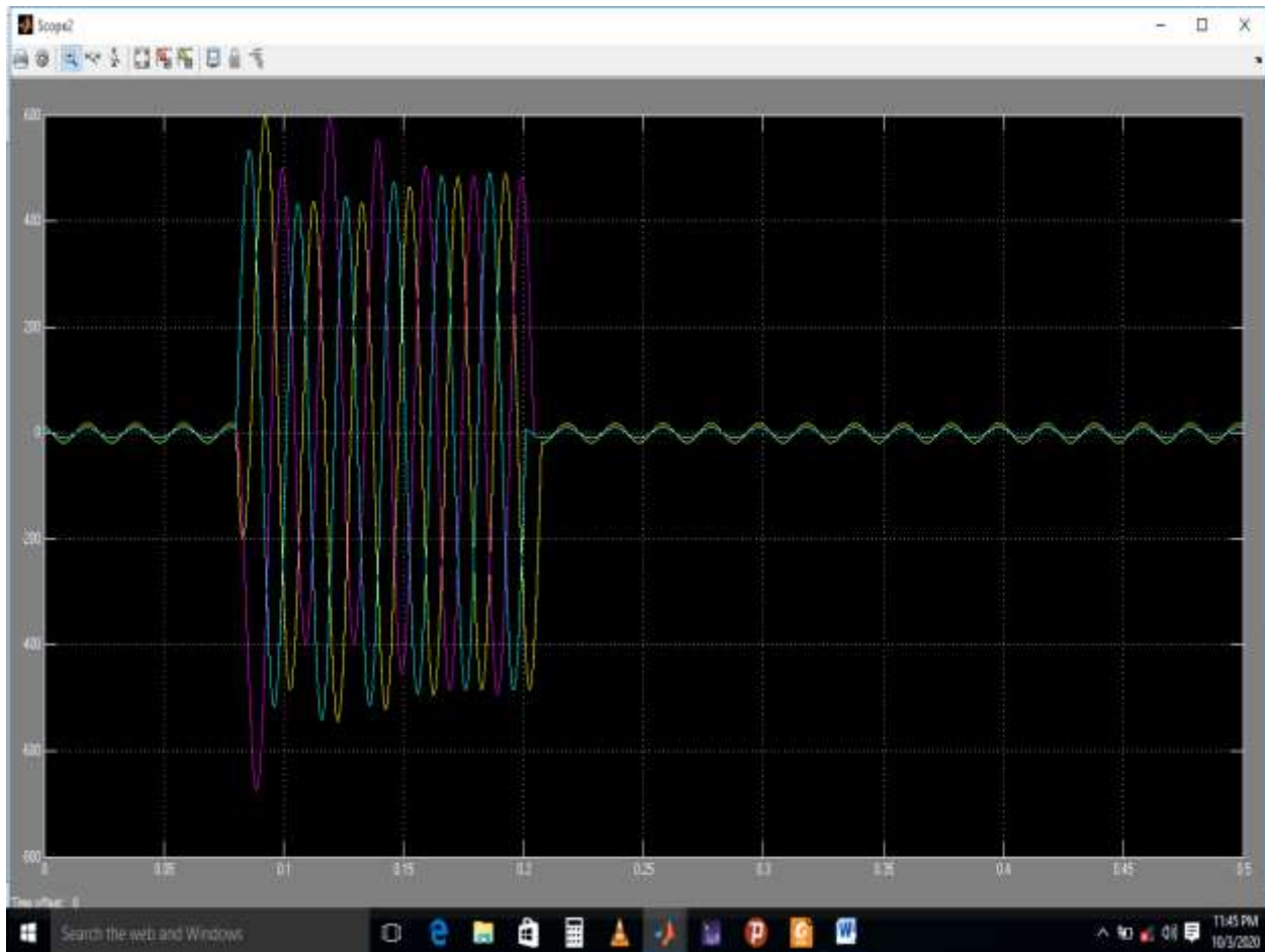
Figure 4.10 Harmonic currents injected by non-linear loads
