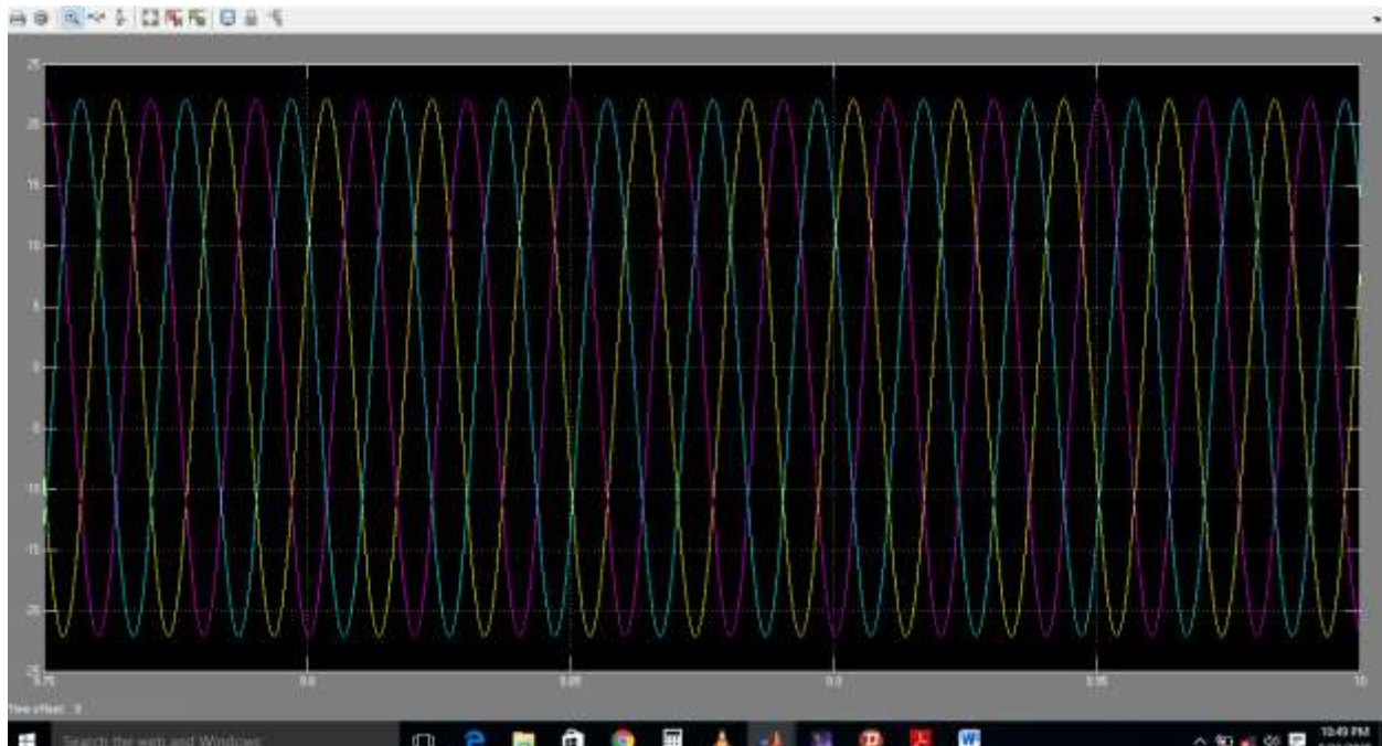
Figure 4.6 Oscillatory transient currents waveform with pre-insertion inductor
