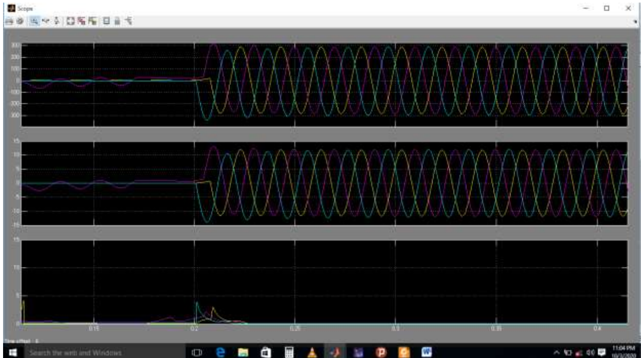
Figure 4.15 Harmonics Mitigation with DSTATCOM
