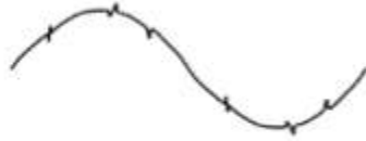
Figure 2.12: Notch wave forms [12].
