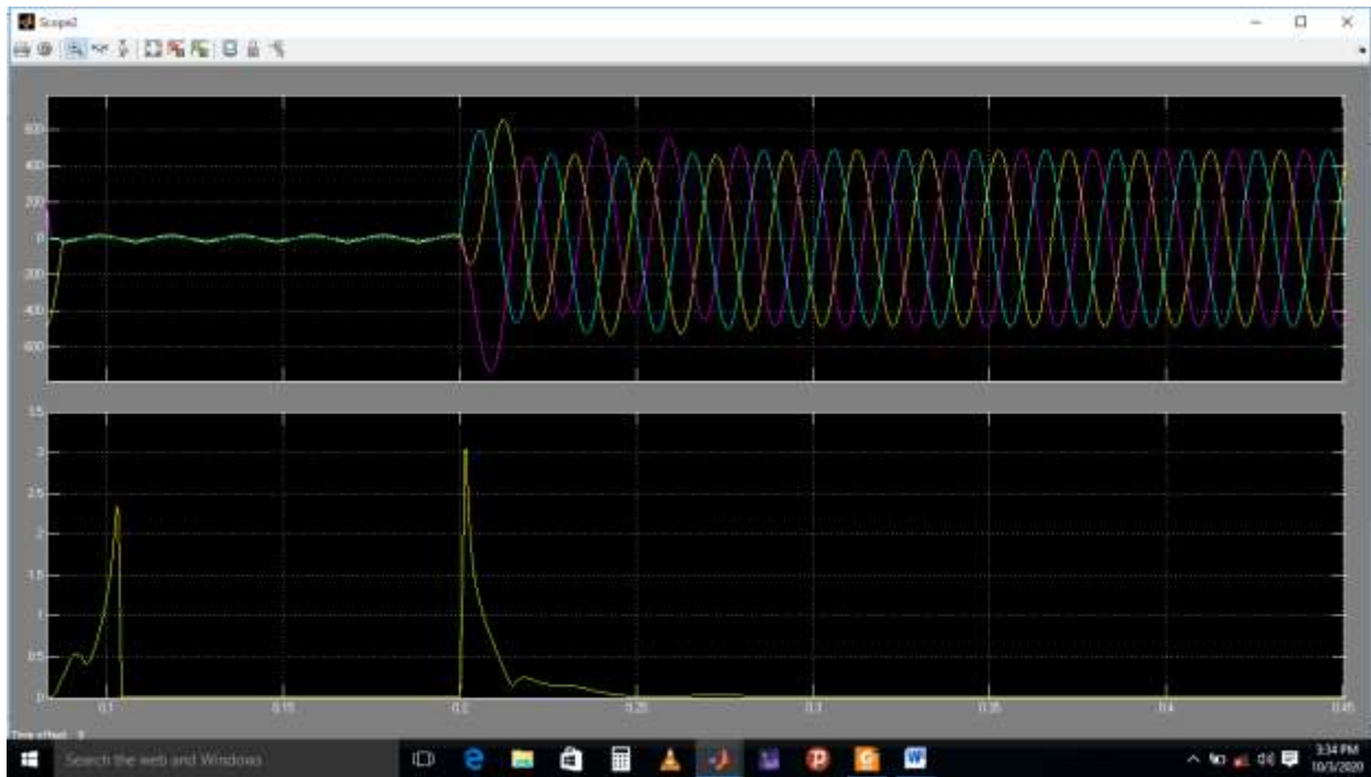
Figure 4.12 Currents waveform and THD with filter
