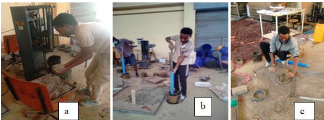
Figure 3.11: Photographs Taken during Compaction Test, a) Adding the material in to the mold b) Compacting the materials c) Trimming the top surface by spatula (Source: Abuye Boja 28/10 /2020)
