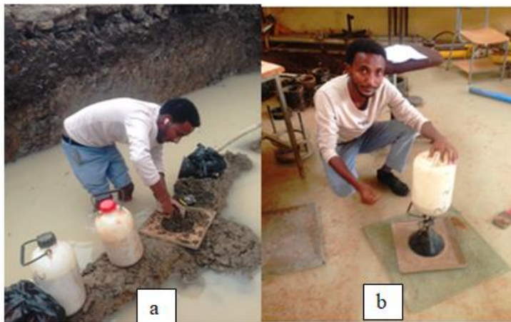
Figure 3.7: Photograph for Field Density Determination a) taking materials at site b) Calibrating the instrument (Source: Abuye Boja 14/10/2020)
