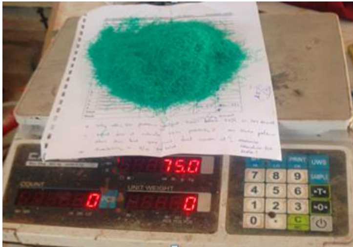
Figure 3.4: Nylon Synthetic Fiber after trimmed in to 10 and 20 mm lengths (Source: The Researcher , 28/11/2020)
