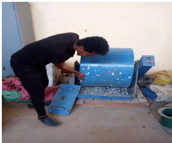
Figure 3. 2 LAA test(photo credit; Dejene D. date Sept 21,2020)
