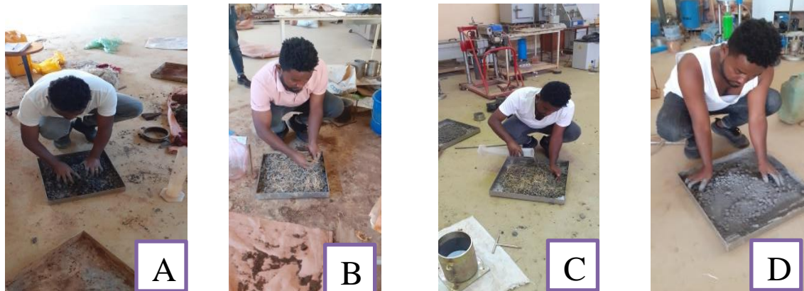
Figure 3. 7: Mixing of soil sample with additives (Source: Ayalew A., 12/3/2013)
