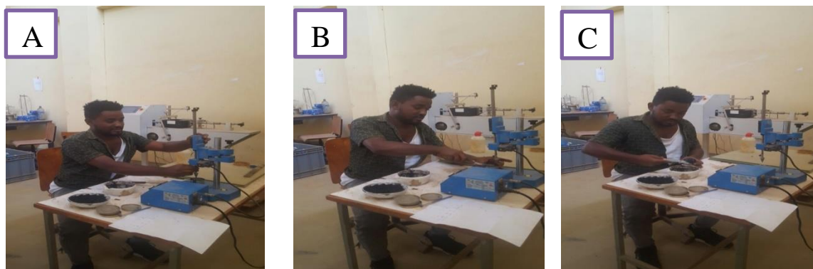
Figure 3.14 : Cone penetrometer test (Source: Ayalew A., 22/4/2013)
