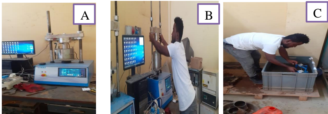
Figure 3. 12: CBR test procedures (Source: Mulukene G., 10/4/2013)
