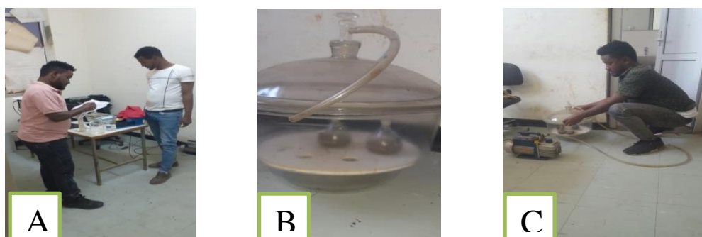
Figure 3. 10: Specific gravity test (Source: Mered H., 1/4/2013)
