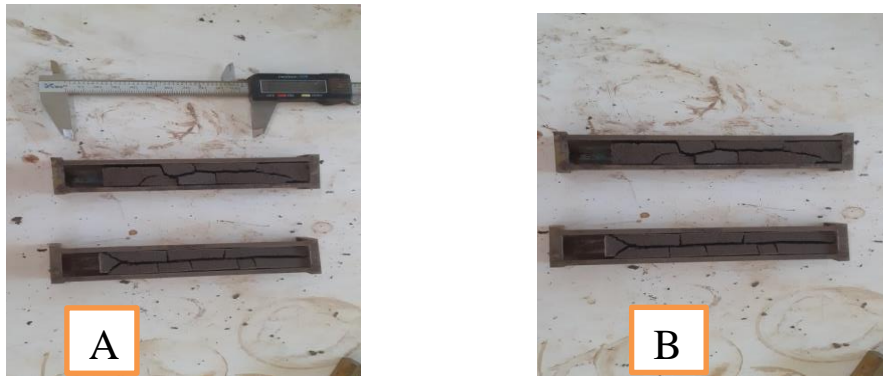
Figure 3. 13: Linear Shrinkage test (Source: Dawit S., 16/3/2013)
