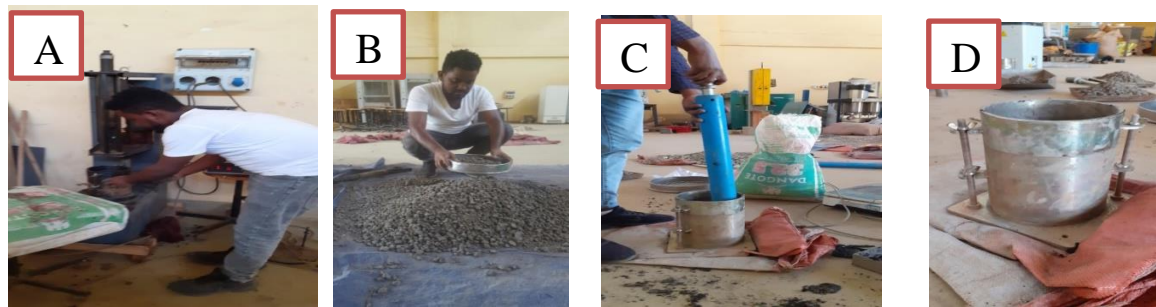
Figure 3. 11: Compaction test (Source: Asbew A., 4/4/2013)
