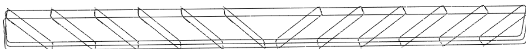
Figure B. 7: 60° inclined stirrups provision in 4m span length of RC beam
