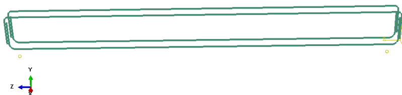
Figure 3. 26: Top and bottom longitudinal reinforcements used in ABAQUS Analysis
