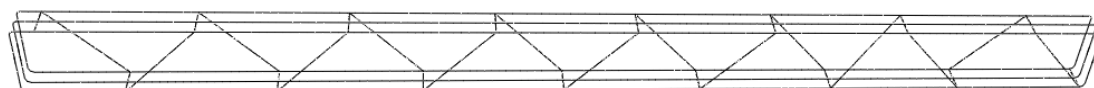
Figure B. 31: 75 0 Rectangular spiral bars provision in 6m span length of RC beam
