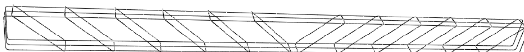
Figure B. 24: 60° inclined stirrups provision in 6m span length of RC beam
