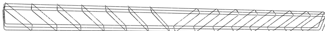
Figure B. 25: 75° inclined stirrups provision in 6m span length of RC beam
