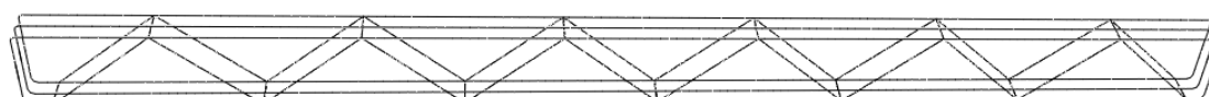
Figure B. 33: 60 0 Warren truss reinforcement's provision in 6m span length of RC beam
