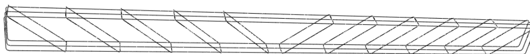
Figure B. 23: 45° inclined stirrups provision in 6m span length of RC beam
