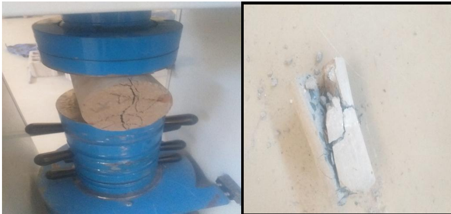
a) Crack pattern during crushing b) Crushed cylinder after peak
