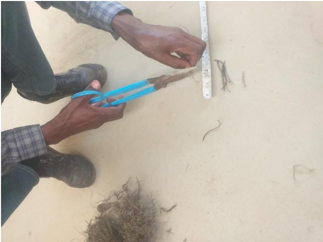
Figure I Photo during length determination for steel fiber
