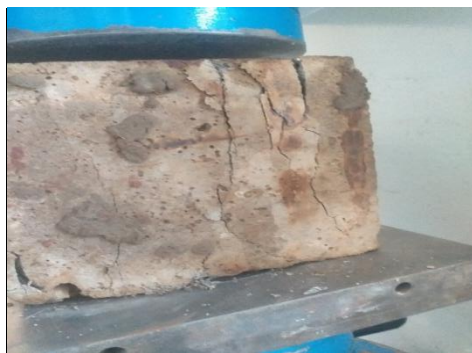
b) crack pattern after crushing
