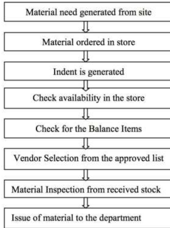
Figure 2 1 Construction Material Management process
