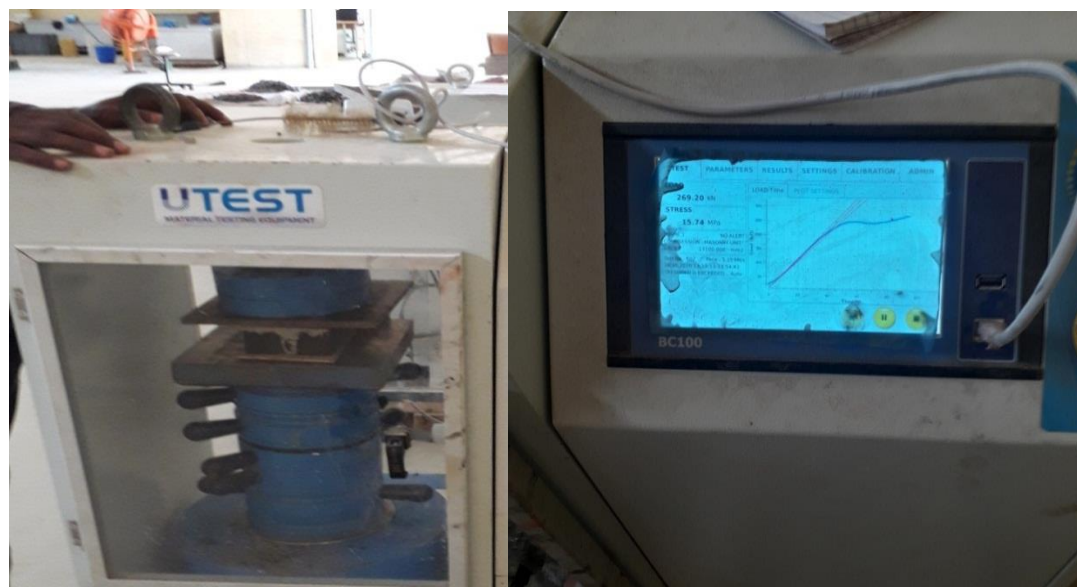
Figure 3.11: Compressive Strength test and result
