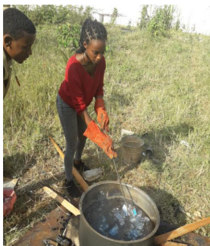
Melting of PET waste plastic
