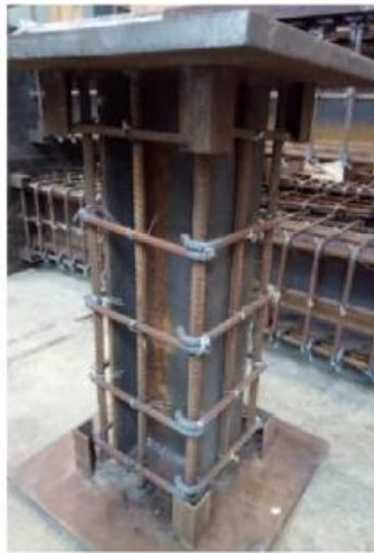
Experiment set up of reinforcements and steel sections
