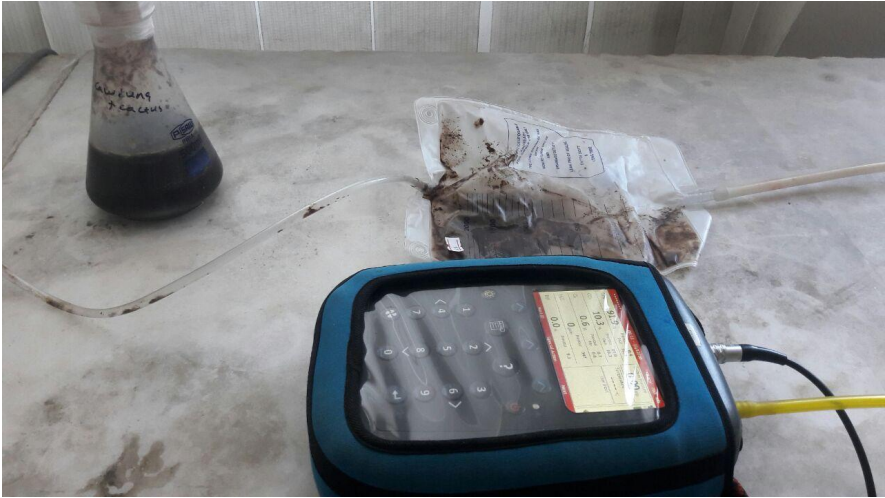
Measuring methane quality by Gas analyzer
