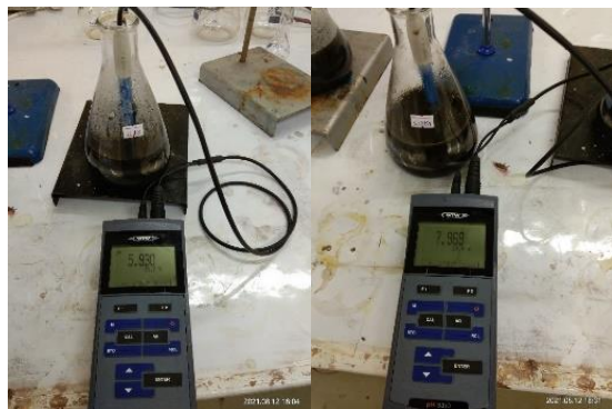
pH adjustment of the solutions during synthesis of ZnO Nps and ZnO-Ag NCs
