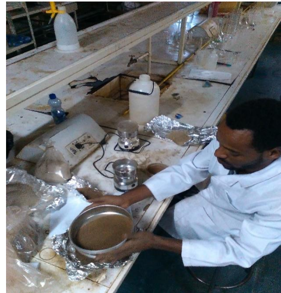
Filtering the HA solution to remove undissolved HA using Pump and 0.45 \mu m filter paper. And Final obtained Humic acid stock solution
