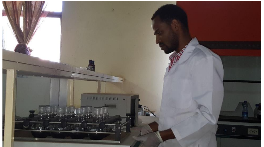
Measuring CACH dose that will be added into the solution and Fixing sample containing Erlenmeyer flask on horizontal shaker.
