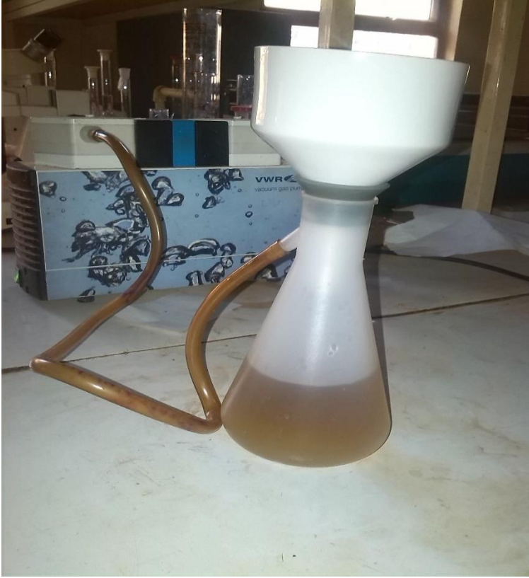
Filtering the HA solution to remove undissolved HA using Pump and 0.45 \mu m filter paper. And Final obtained Humic acid stock solution
