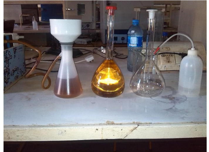
Filtering the HA solution to remove undissolved HA using Pump and 0.45 \mu m filter paper. And Final obtained Humic acid stock solution
