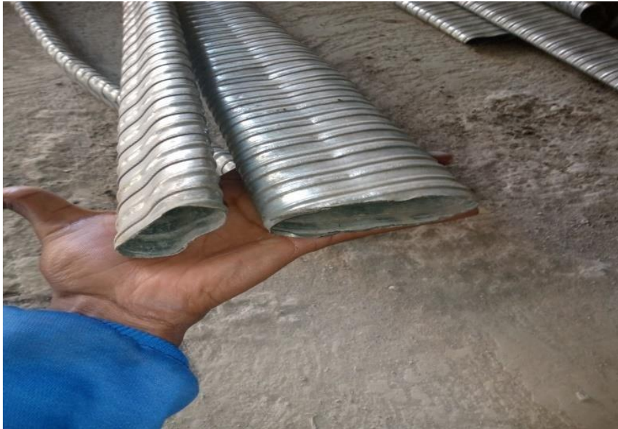
Figure4.9 Duct of 55 and 65mm diameter
