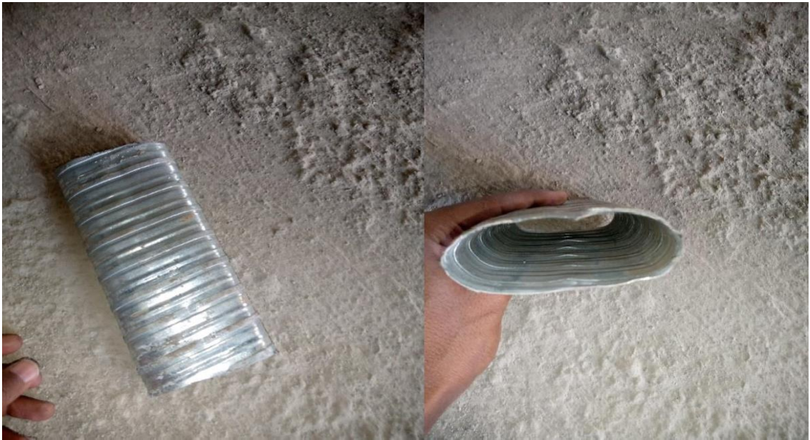
Figure4.15 connector/coupler 70mm diameter
