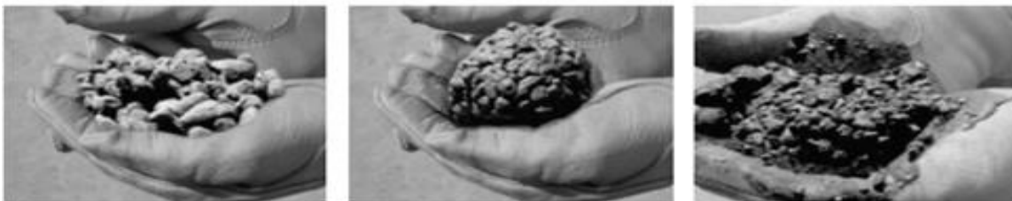
a) Small water content b) Optimum water content c) Optimum water content
