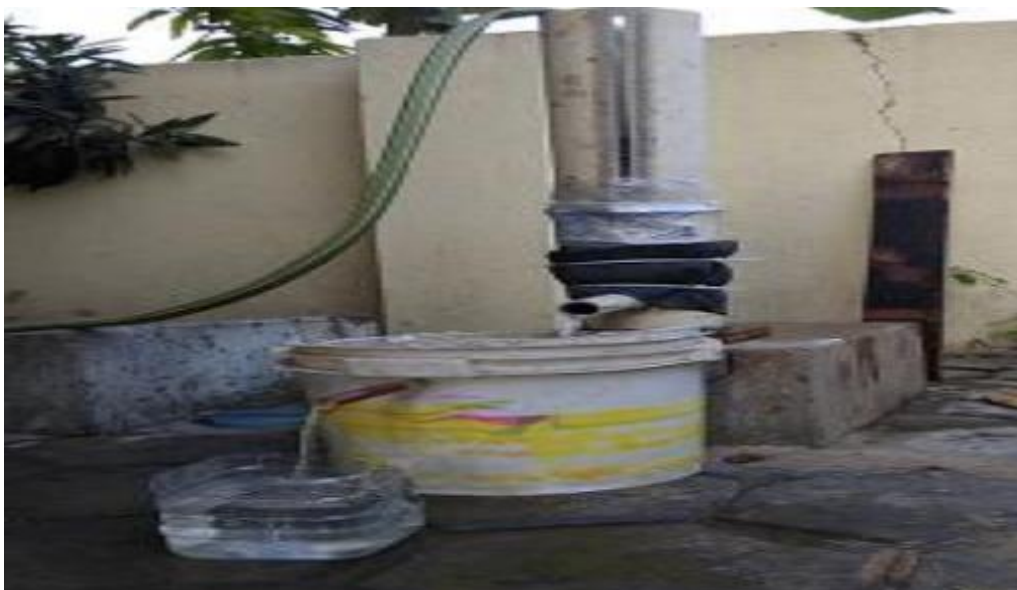
Figure 2.7: Test setup for constant head method
