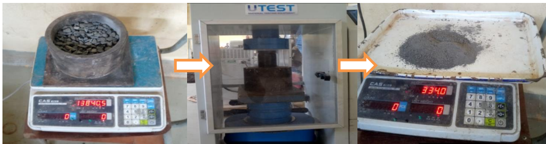
Figure 3. 12 Aggregate crushing value determination processes
