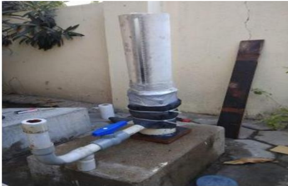
Figure 2.6: Test setup for falling head method
