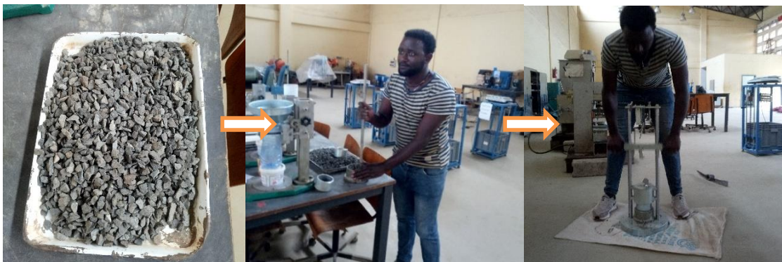
Figure 3. 11 Aggregate impact value test
