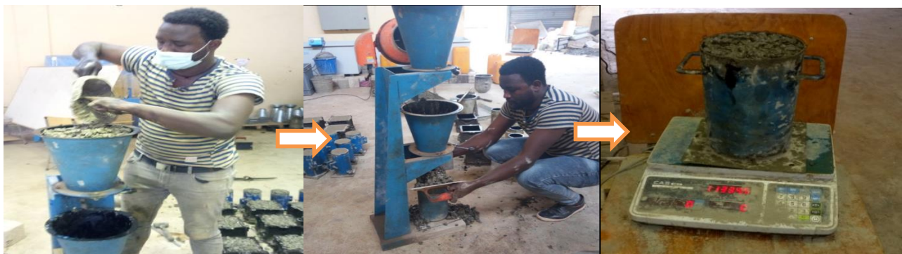
Figure 3. 16 Compacting factor test processes
