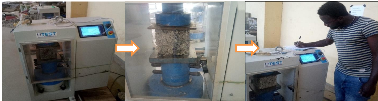
Figure 3. 18 Compressive strength determination using a universal testing machine
