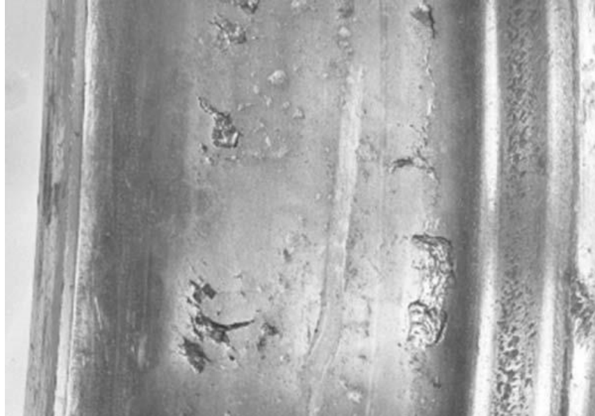
Figure 2.4 Wheel surface fatigue damage
