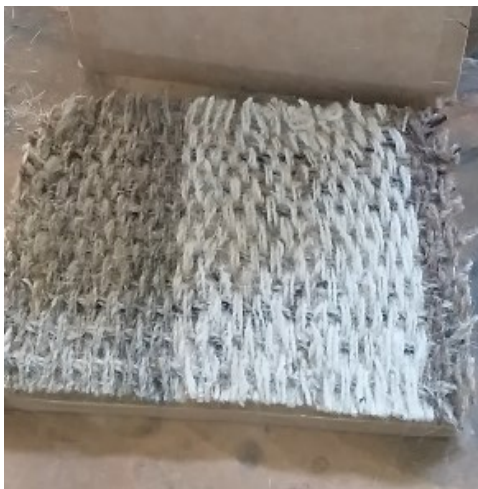
Figure 3.6 Composite material preparation a) cutting the woven fiber with mold dimension and b) pouring of epoxy into the fiber
