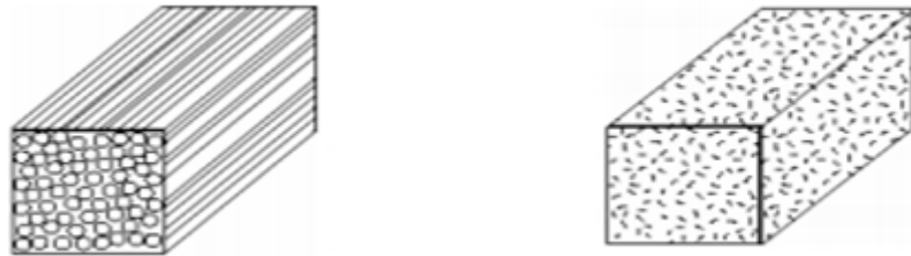
Figure 2.4 Fiber with a) Continuous longitudinal oriented fiber and b) Random oriented chopped fibers [32].
