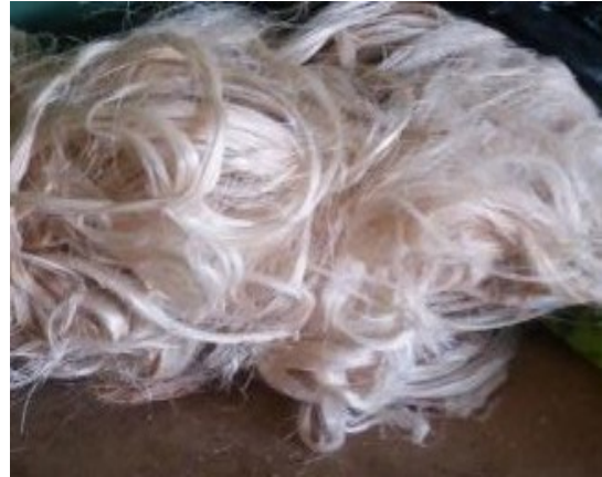
Figure 3.3 a) Manual extraction of Enset fiber and b) Enset fiber
