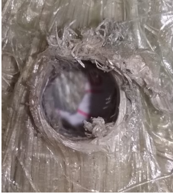
Figure 4.26 Drilled hole front and backside
