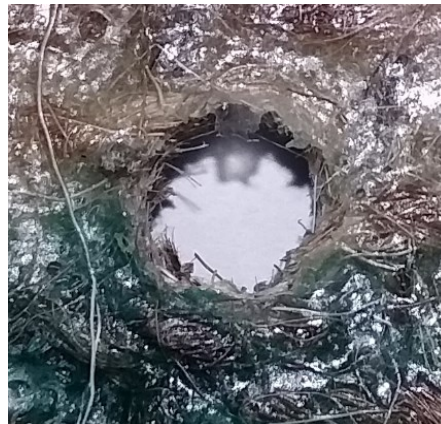
Figure 4.27 Drilled WEW, MMM with 50% fiber volume ratio HFCM
