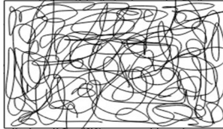
Figure 3.10 Random continuous fiber orientation
