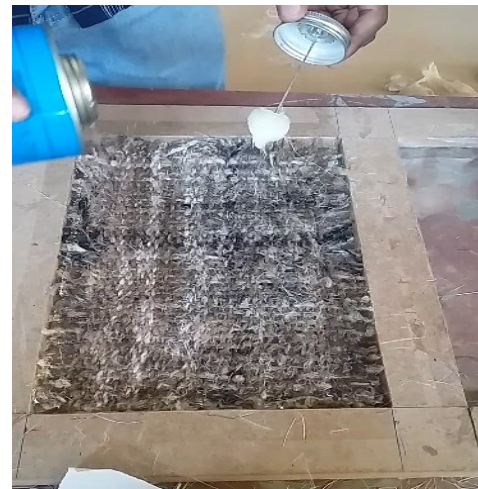
Figure 3.6 Composite material preparation a) cutting the woven fiber with mold dimension and b) pouring of epoxy into the fiber
