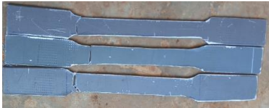
Ductile failure of sandwich sheets.
