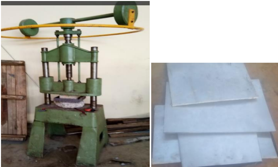
Figure 3. 3 : a) manual spindle pressing machine b) Three kinds of sandwich sheet products
