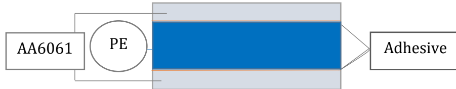
Figure 3. 1: Schematic of the layup of the AA6061/HDPE/AA6061
