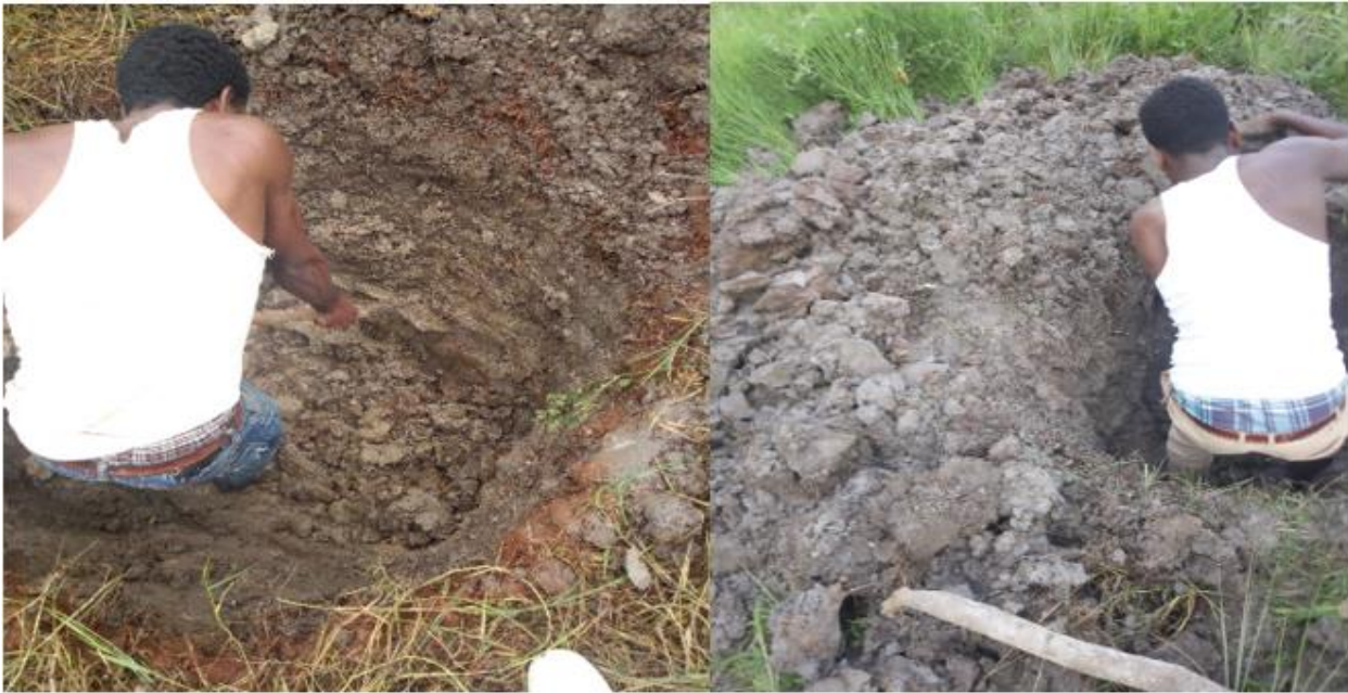
Figure 1 Excavated test pits
