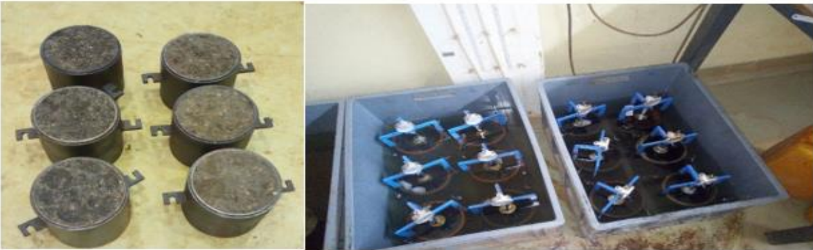
Figure 6 compacted sample and soaked sample for CBR test.
