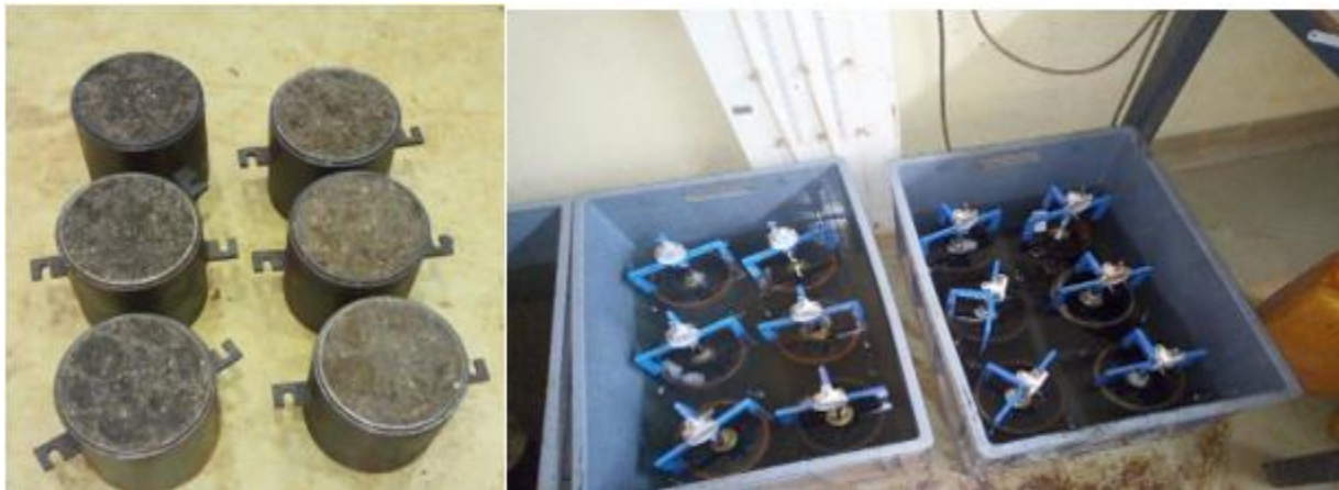
Figure 3.8 compacted sample and soaked sample for CBR test.
