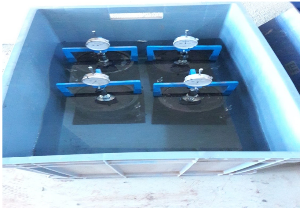
Figure A13: Photo taken while soaking BC soil for CBR test
