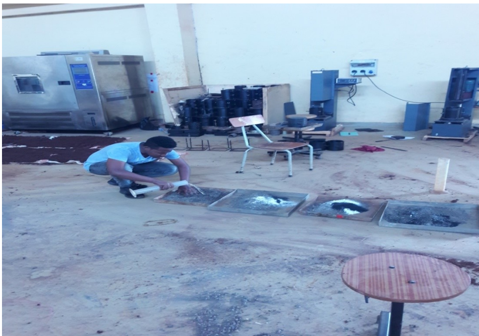
Figure A7: Mixing a BC soil with mixtures for the modified compaction
