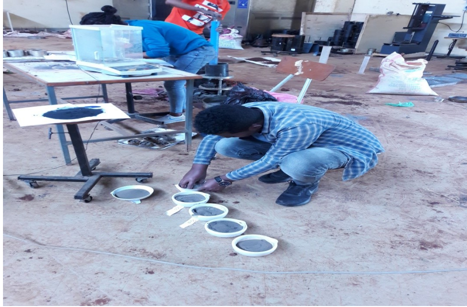
Figure A8: Soaking and mixing A BC soil with lime and corncob for the atterberg limit
