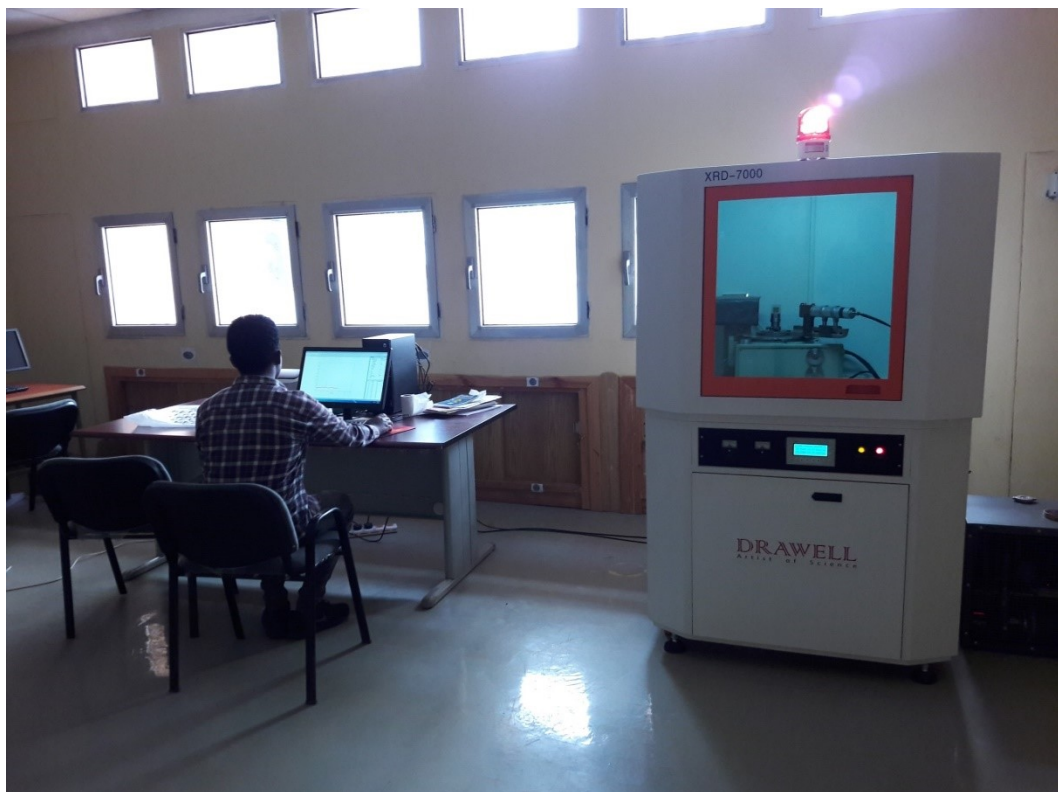
Figure A4: Photo taken during testing the mineralogy of the mixture by XRD
