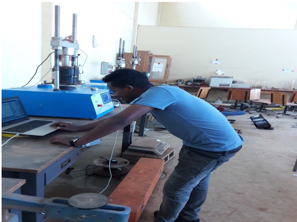
Figure A15: Photo taken while setting up a software for CBR penetration
