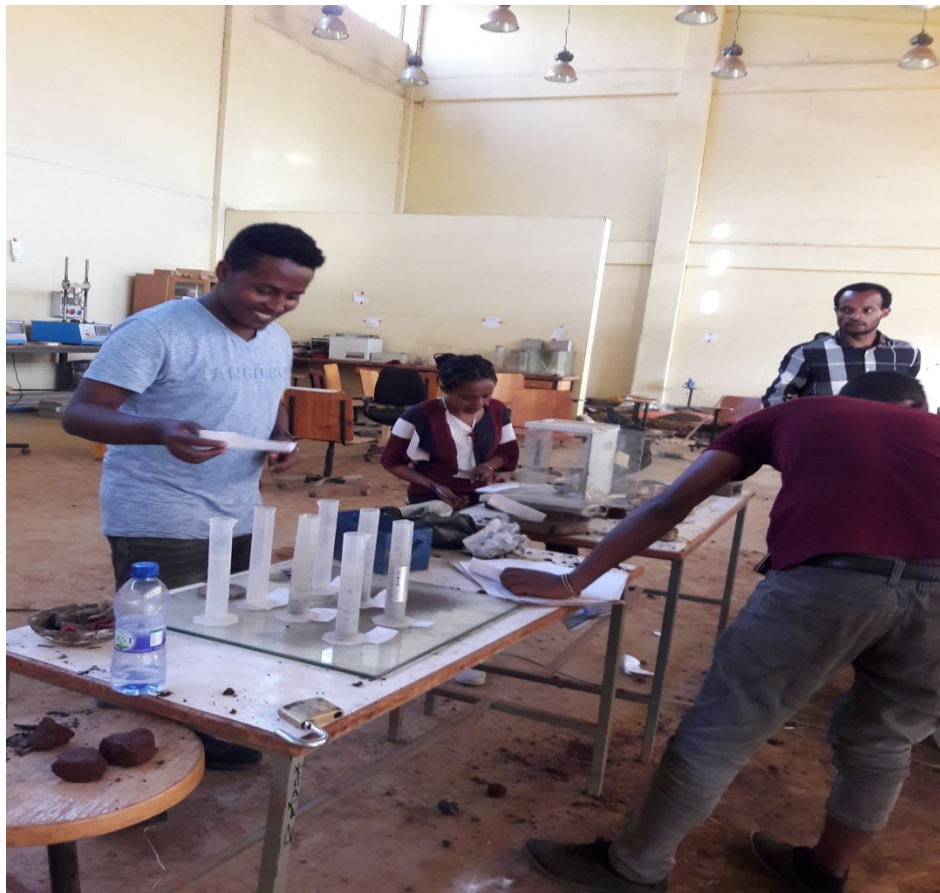
Figure A9: Preparing a BC soil with mixtures for free swell index
