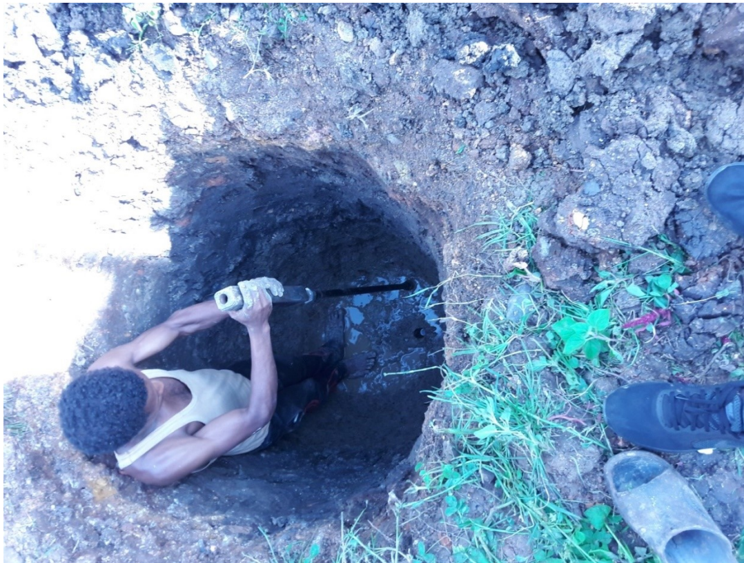
Figure A2: Photo taken during taking undisturbed BC soil sample
