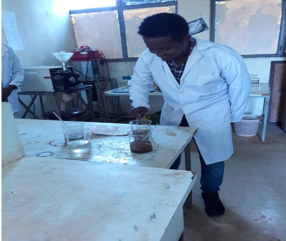
Figure A12: photo taken while mixing BC soil with sodium hexa methaphosphate
