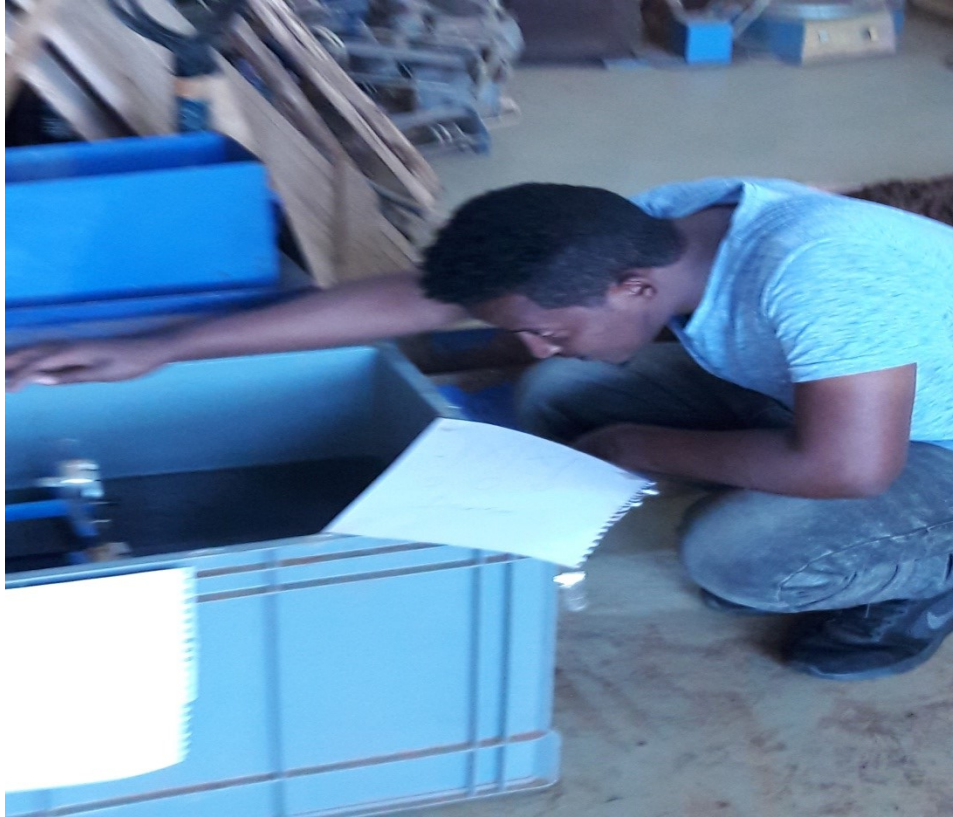
Figure A14: Photo taken while reading CBR swelling
