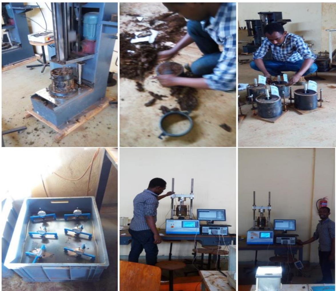
Figure 3.8: Apparatuses for CBR test
