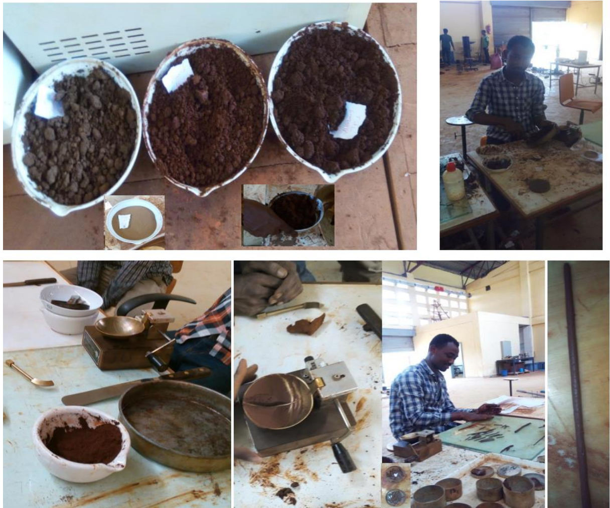
Figure 3.6: Apparatuses for atterberg's test
