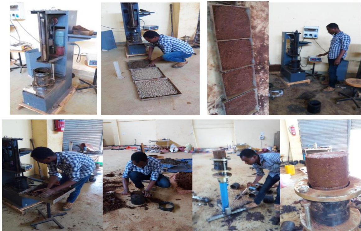
Figure 3.7 Apparatuses for a compaction test
