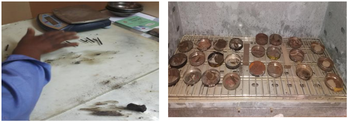
Figure 21 Plastic Limit test and Samples of LL, PL and Ls test during oven drying (Source: photos taken during Plastic Limit test and samples of LL, PL & Ls inside an oven)
