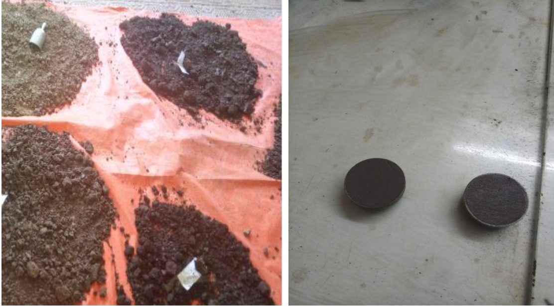
Figure 18 Disturbed samples and undisturbed samples (Source: photos taken of the samples in the laboratory)
