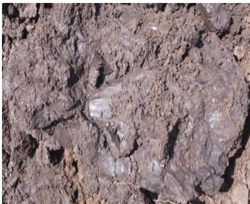
Figure 6 Wet slippery expansive soil sample and Desiccation cracks( Source; Photos taken while sampling and visual identification)
