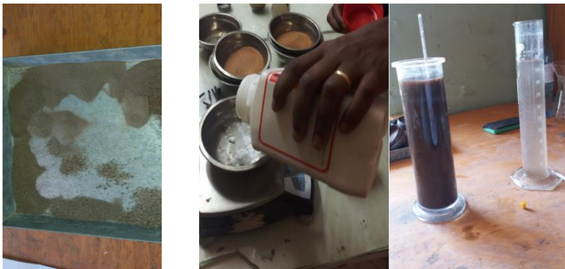
Figure 23 wet sieve analysis result and Hydrometer Analysis (Source: photos taken after wet Sieve and during hydrometer analysis)
