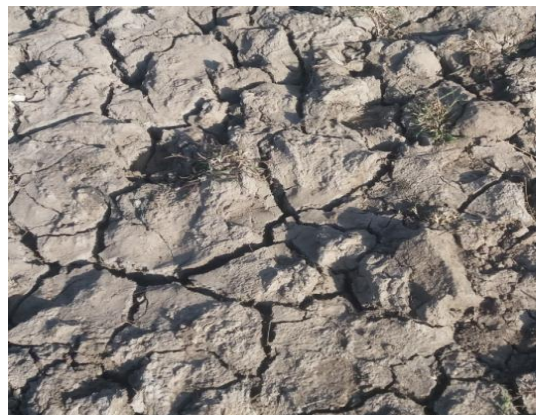
Figure 6 Wet slippery expansive soil sample and Desiccation cracks( Source; Photos taken while sampling and visual identification)
