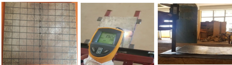
Fig. 1. Measurement of sheet metal temperature & deformation.
