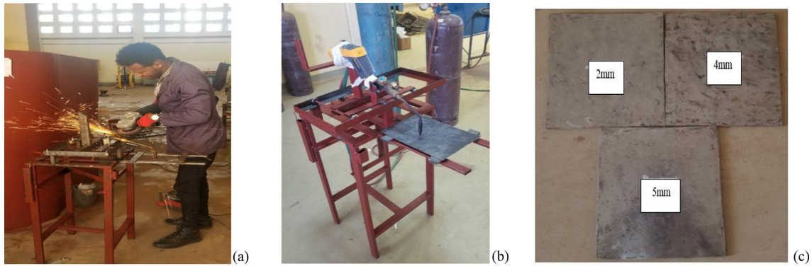
Fig. 16. (a) Set up for the experimental investigation, (b) position of the sheet metals; (c) sheet metal with different thickness.
