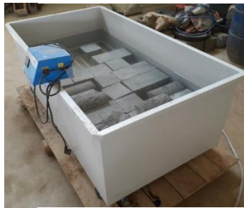
Curing of concrete
