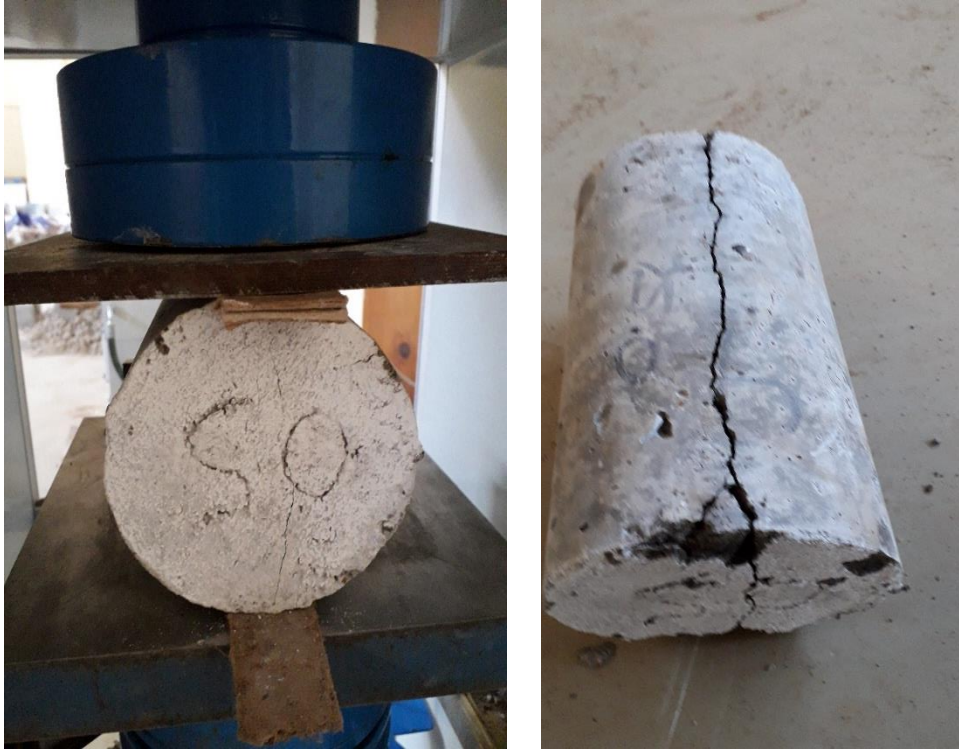
FIGURE A-6. Failure mechanism for 0.5 % SFRC under splitting tensile test
