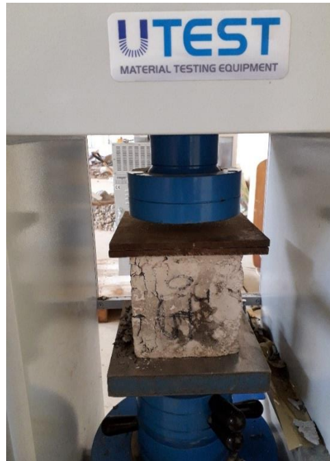
Figure A-5. Failure mechanism of 0.5 % SFRC under compression test
