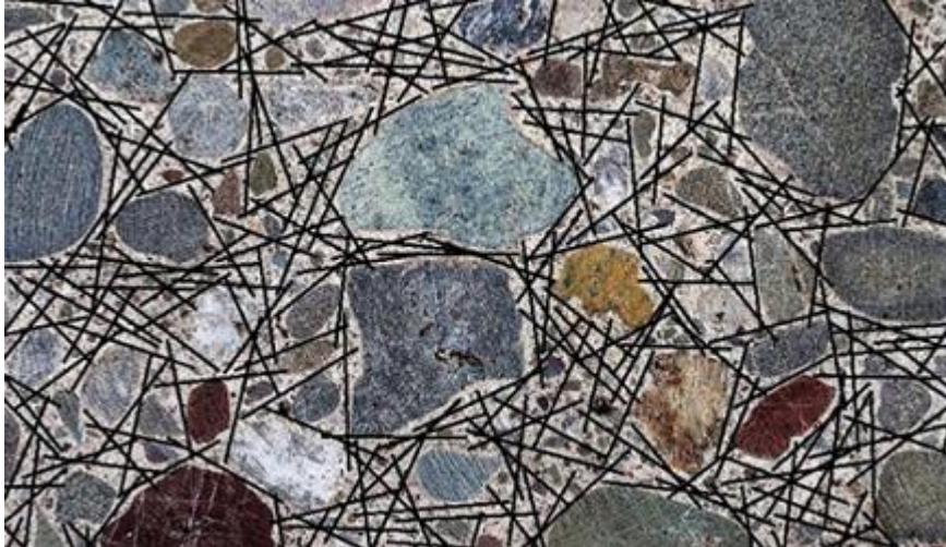
FIGURE 2–2. Steel fiber reinforced concrete section (Singh, 2017).
