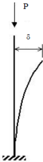
Figure 2.13 P- \delta effects on a column [2]
