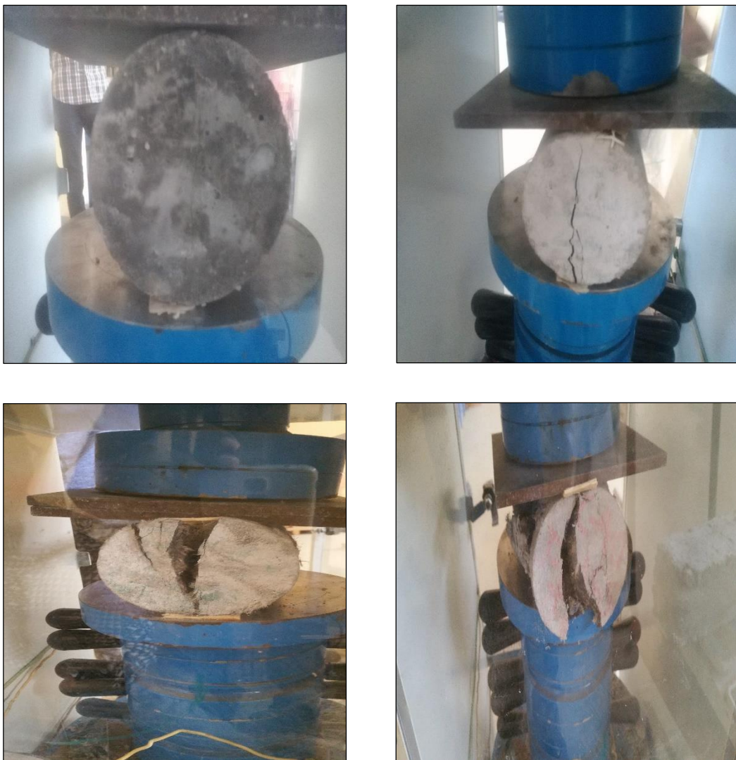
Figure 3-5 Split tensile test; a) test setup; b) first crack initiation; c) near to failure ;and d) at failure stage
