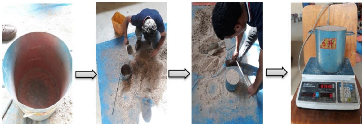
Figure A-3: Unit weight determination of fine aggregate
