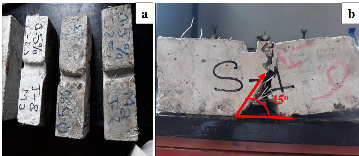
Figure 4-12 Shear strength test ;a)Specimen prepared for test ; and b) Failure pattern (crack angle) of a macro synthetic beam under shear test
