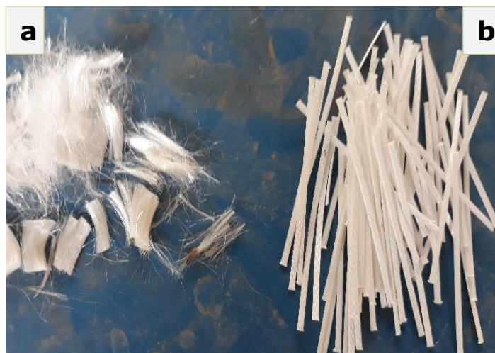
Figure 3-2 Synthetic fibers: a) Micro virgin polypropylene synthetic fiber; b) Macro polypropylene synthetic fiber
