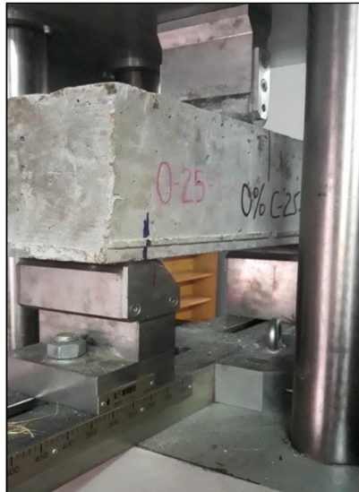
Figure 3-6 Flexural strength test under loading
