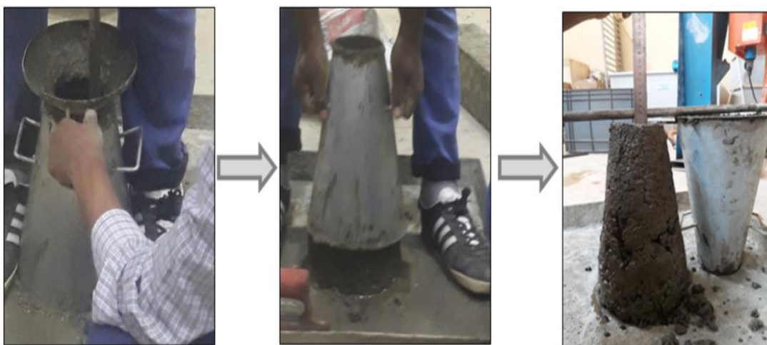
Figure 4-1 Steps in filling concrete cone and slump height measurement
