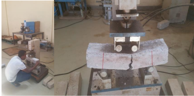
Figure 3.12 Flexural strength testing
