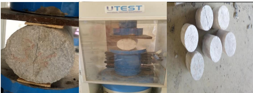
b. Cylinder crack
