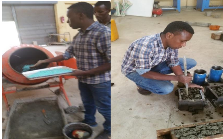
Figure 3.4 Adding of replacement HDPE in concrete mix and compacting the mix in the mould
