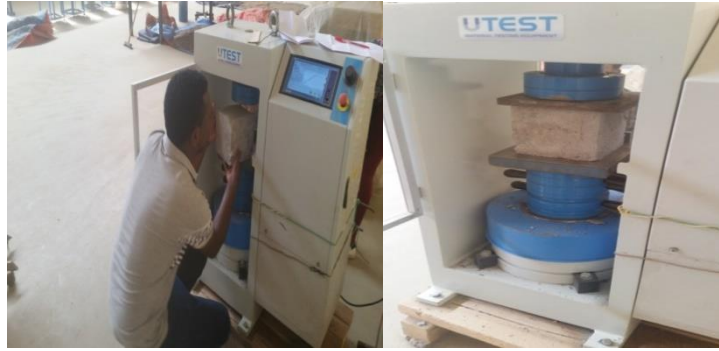
Figure 3.8 Compressive strength test using compressive testing machine
