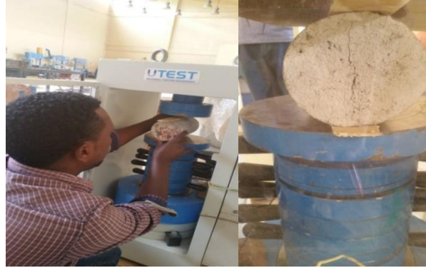
Figure 3.10 Split tensile strength testing
