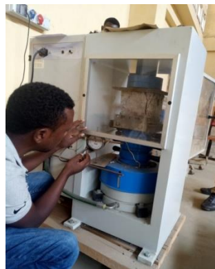
Figure 3.9 Strain gauge for cube compression test
