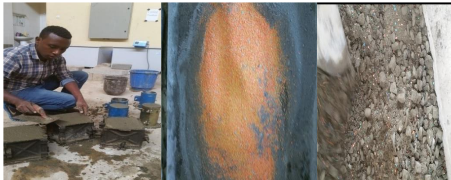
Figure 3.5 Homogeneously mixing of aggregates and surface finish of sample in moulds during casting.
