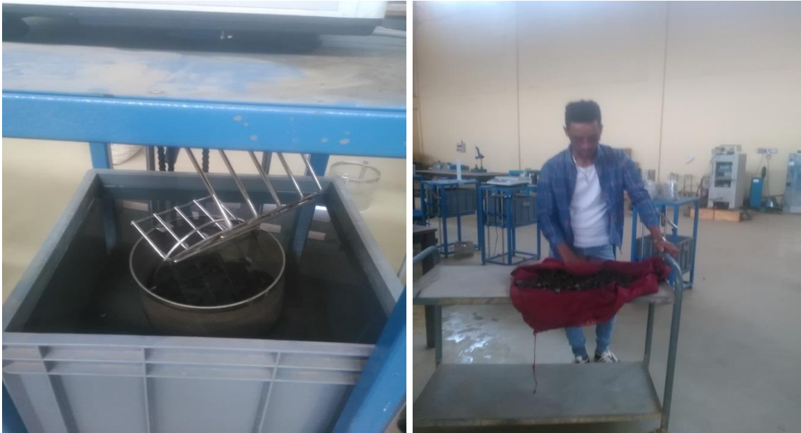
Picture-1: Soaking and surface drying of coarse aggregate for specific gravity test
