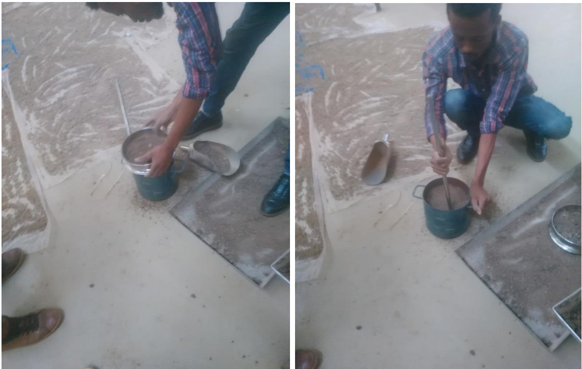
Picture-4: Preparing fine aggregate for unit weight test
