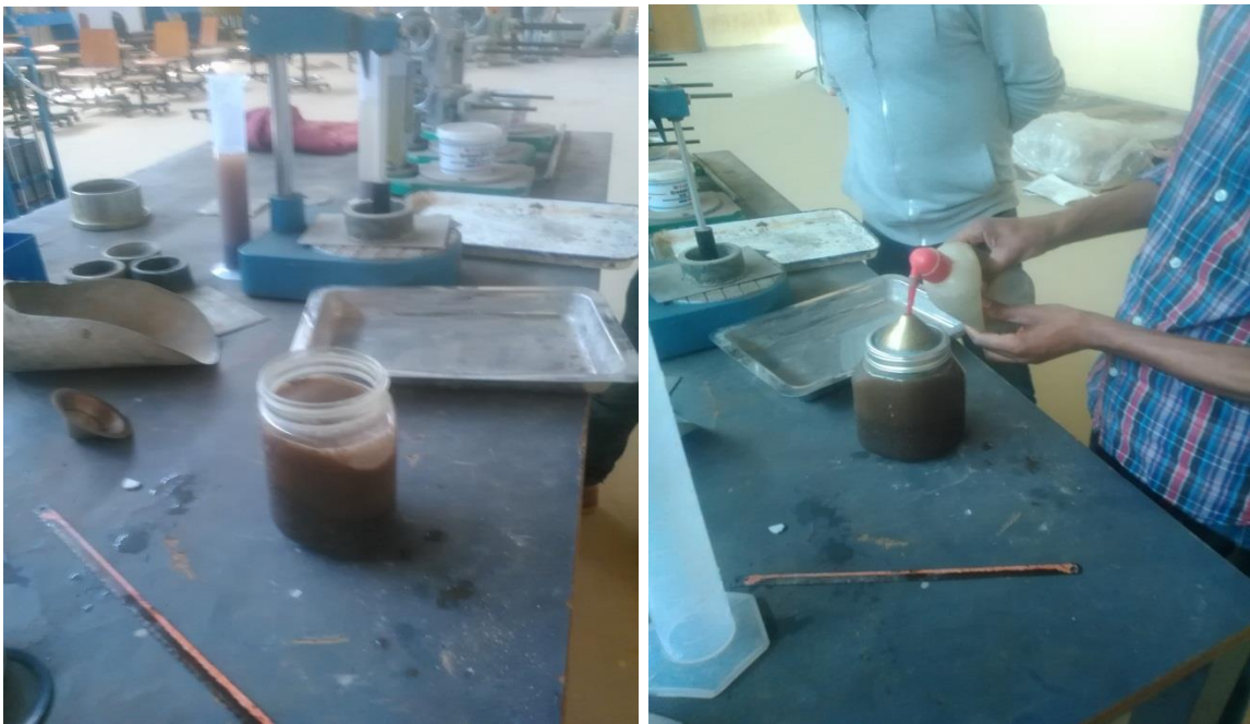
Picture-2: Specific gravity test for fine aggregate
