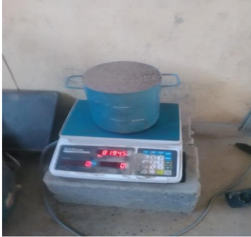
Figure 3.5 Unit weight test of fine aggregate
