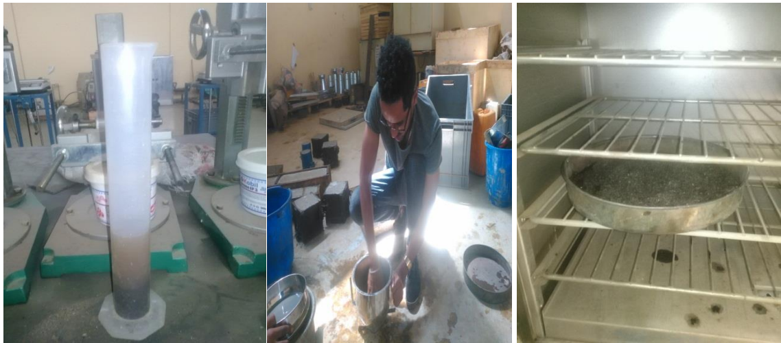
A, Silt content test using tube B, Washing the sand C, Oven drying the sand
