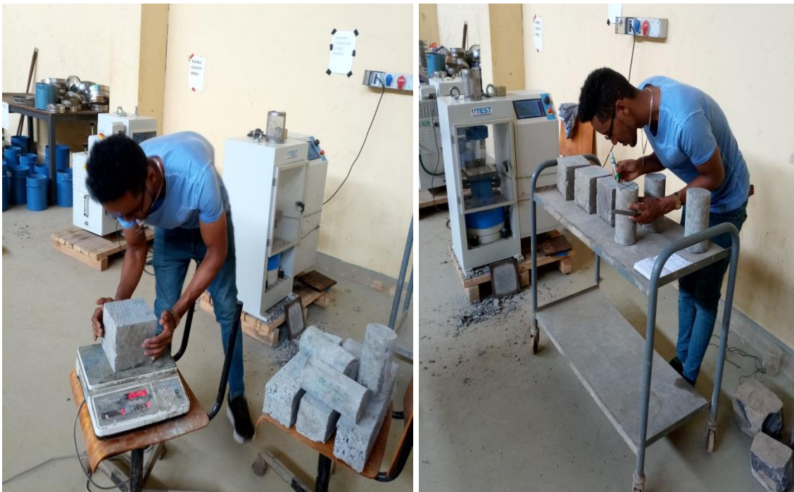
A, Measuring the weight of the specimen B, Drawing center line a light on specimen
