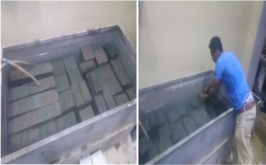
Picture-13: Curing of concrete specimens in tank
