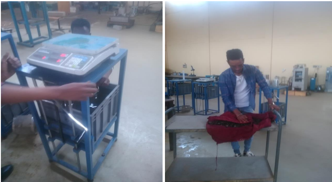
A, Soaking of coarse aggregate in water B, Surface drying of soaked aggregate
