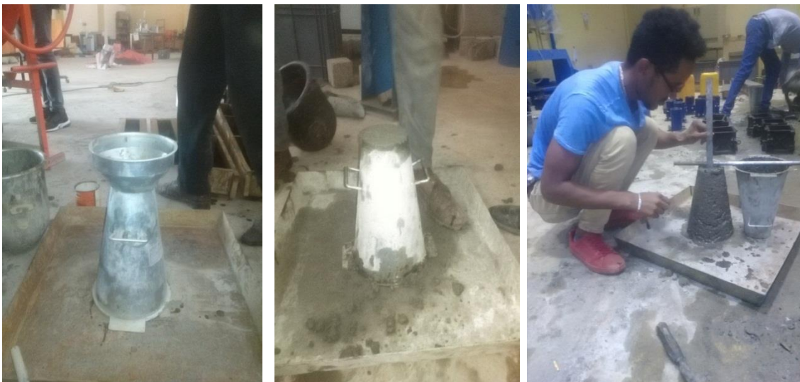
Figure 3.12 Workability test of fresh concrete
