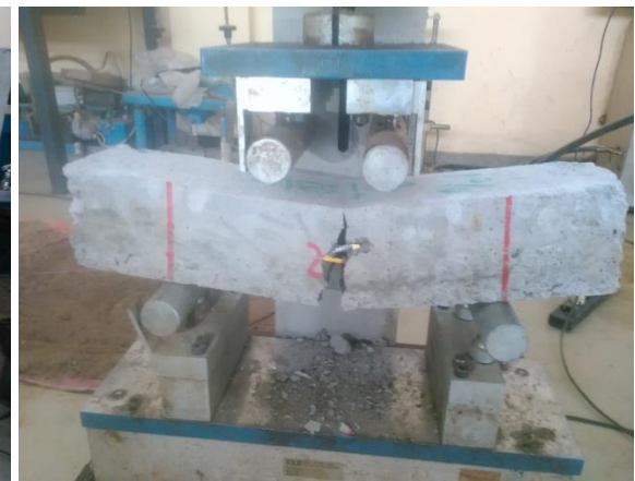
F, 1% SBCF concrete
