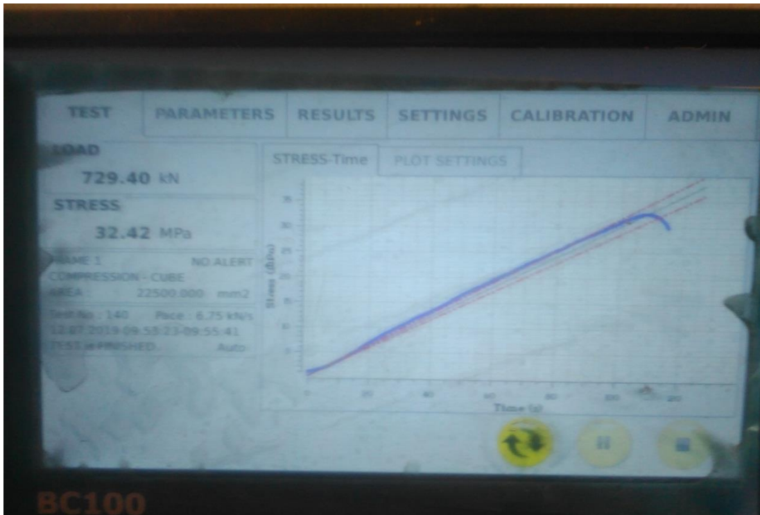
Picture-16: 0% SBCF Compressive test (load (KN) vs. time (s) graph)
