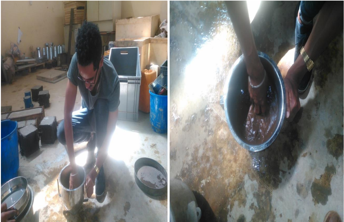
Picture-5: Washing of sand to check its silt content
