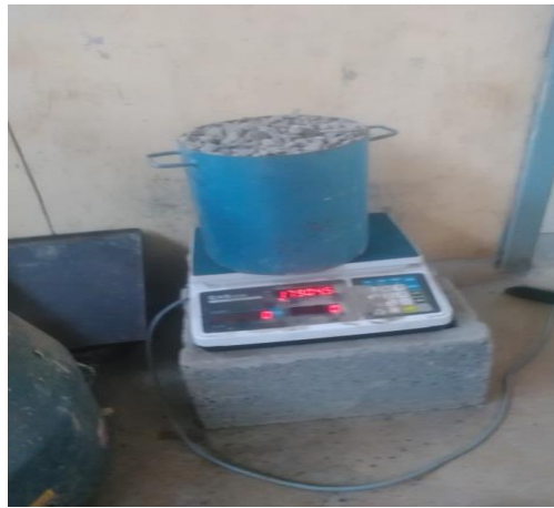
Figure 3.6 Unit weight test of coarse aggregate
