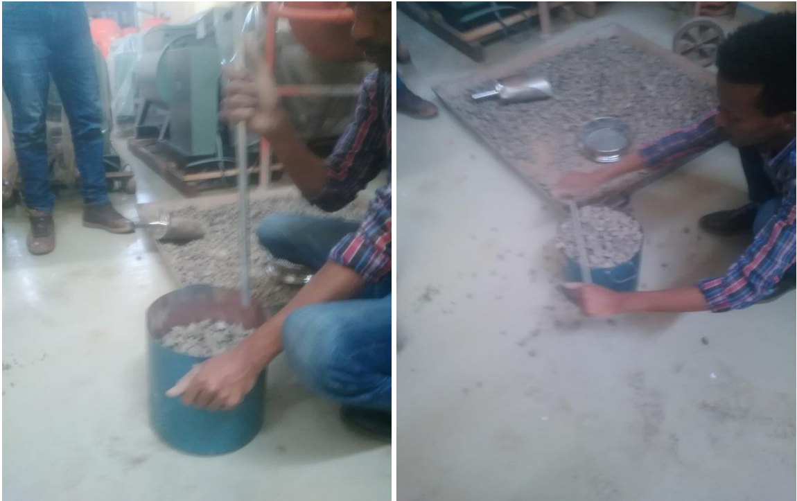
Picture-3: Preparing coarse aggregate for unit weight test
