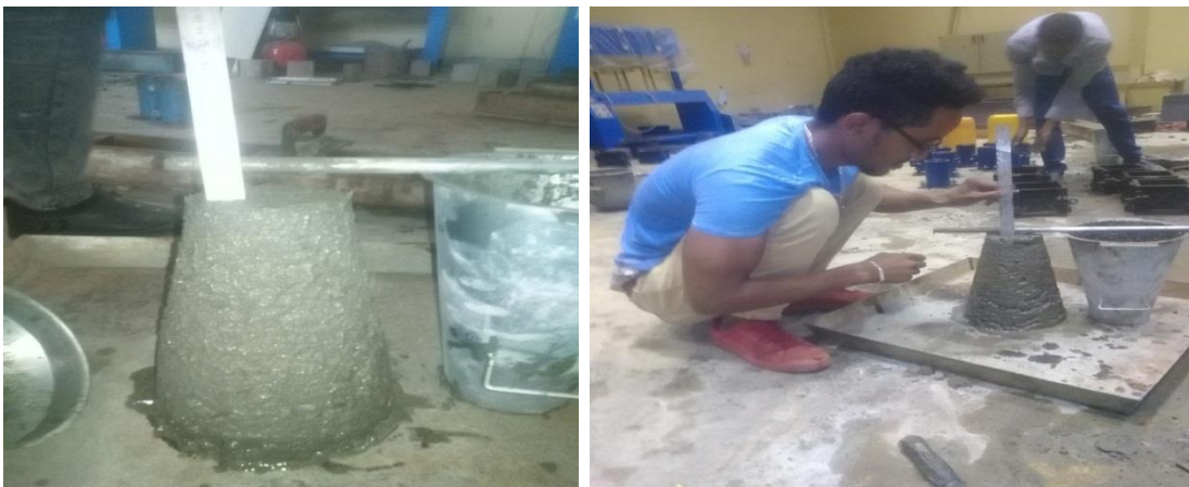
C, 0% SBCF concrete slump
