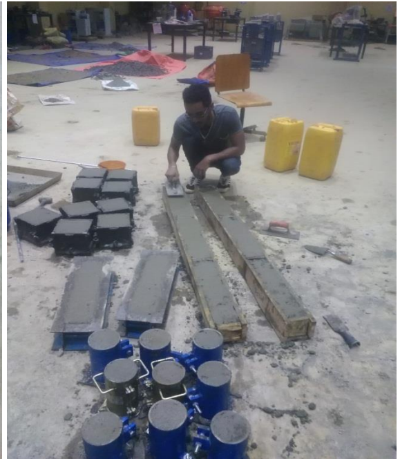
B, Casting of concrete specimen
