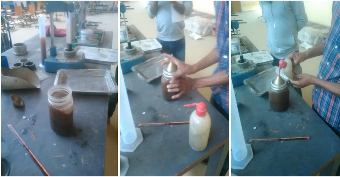
Figure 3.8 Specific gravity test of fine aggregate
