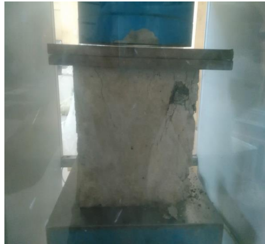
A, JiT compressive test machine (UTEST) B, Cube test
