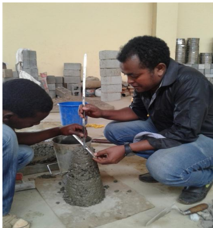
Figure 4.4: Slump test in civil engineering laboratory (Photo taken by Merid Teshome)
