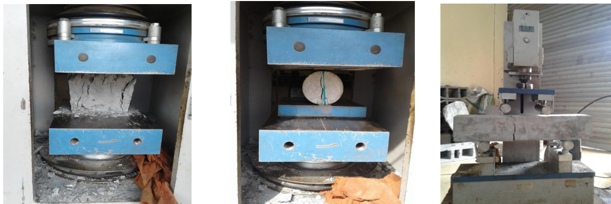
Figure 4.5: The strength tests for compressive, tensile and flexural respectively (Photo taken by Merid).
