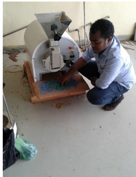
Shredding and cutting of PET (Photo taken by Merid Teshome)
