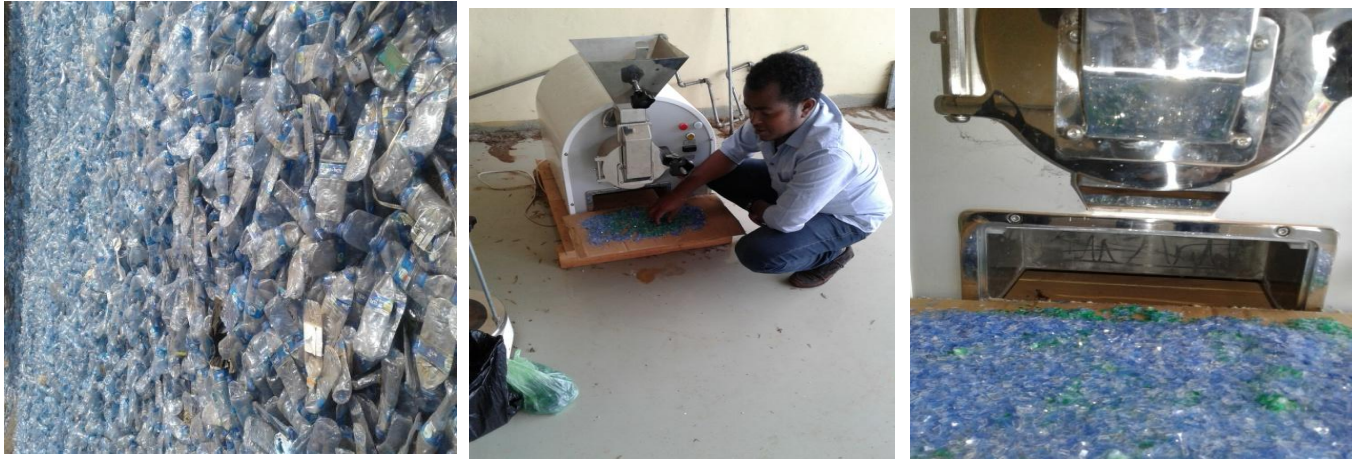
Figure 4.3: Size reduction of PET plastic waste bottles to river sand size (2mm) at chemical engineering laboratory (Photo taken by Merid Teshome).
