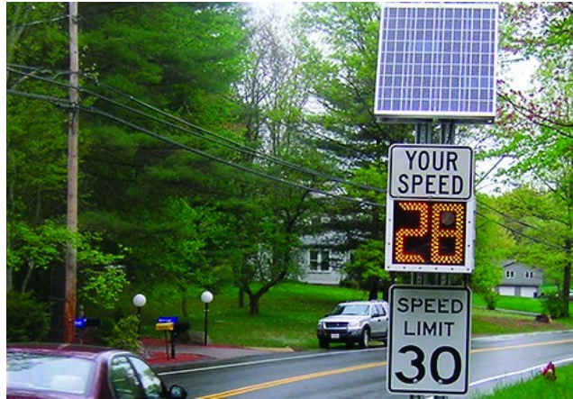
Figure 2.6 a solar-powered speed feedback sign (Source: Evaluation of Gateway and Low Cost Traffic-Calming Treatments, 2007).
