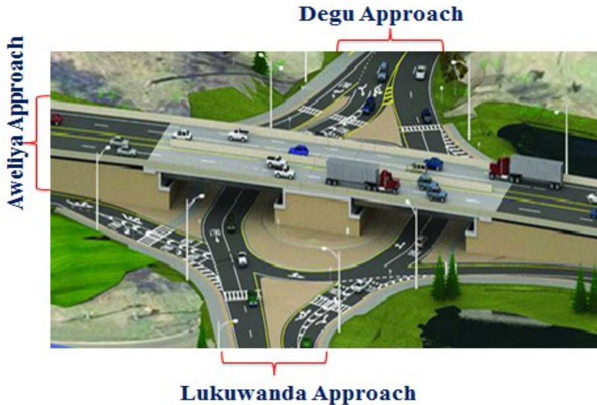
Figure 4.31 Sketch of Asrasimint road section after recommended improvement using Software (Google SketchUp Pro 8.)
