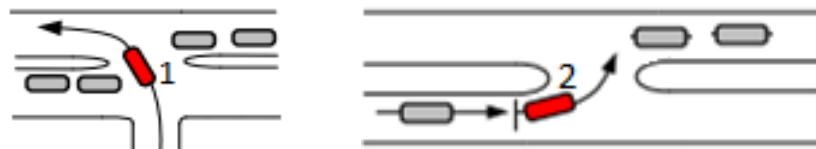
Figure 4-20: Two Types of Conflicts Caused by the Narrow Median Width.
