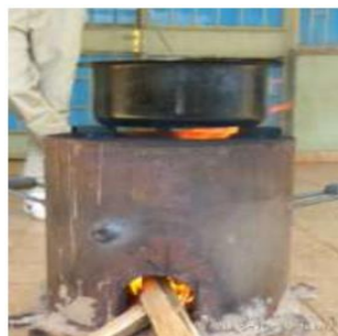
Figure.3.10 producing biochar in continuous feeding anila stove.
