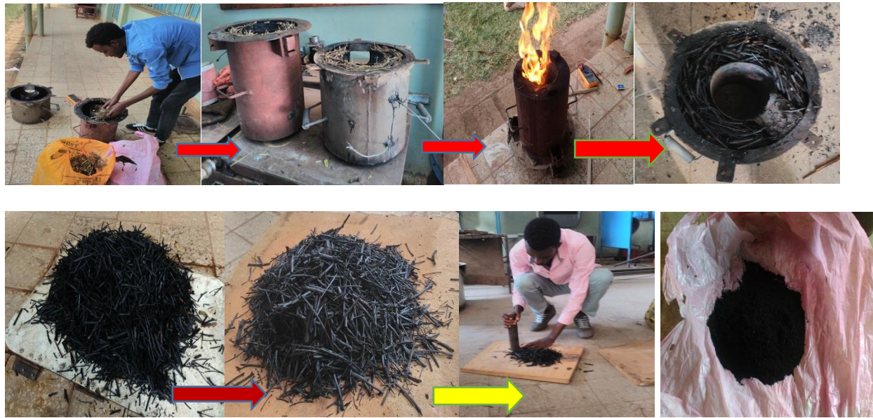
Figure 3.7. Biochar produced in Normal Anila and Continuous feeding Anelia stoves
