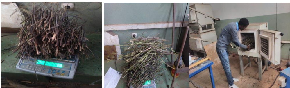
Figure 3.1 measuring the moister content of the khat.
