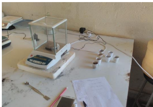
Figure 3.2 .measuring biochar to determine the ash content.
