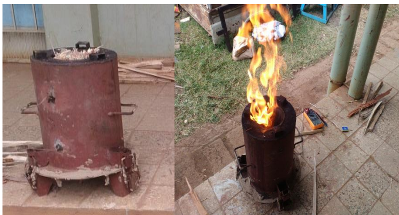
Figure 3.9 producing biochar in normal Anila stove
