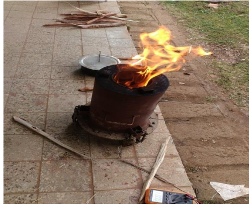
Figure 3.6 Water boiling test in normal feeding Anila stove
