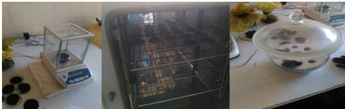
A, Mass balance. B, heating biochar in furnace c, putting the heated char in desiccator
