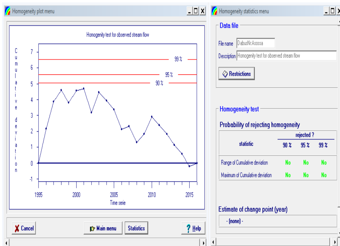
Figure 3.8: Homogeneity test of flow data
