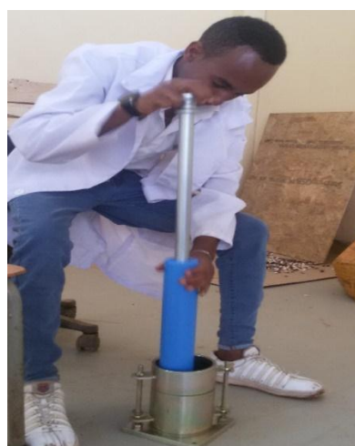
Fig.2: Pestle for corn cob crush
