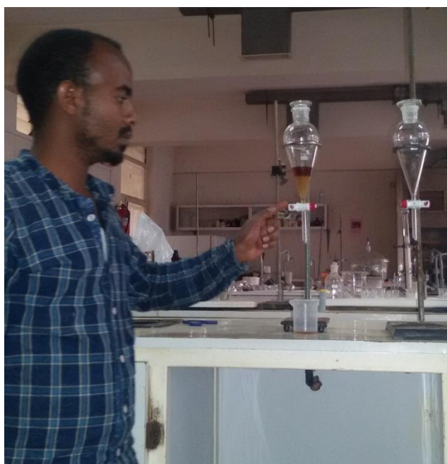
Figure : Separation process of biodiesel and glycerol
