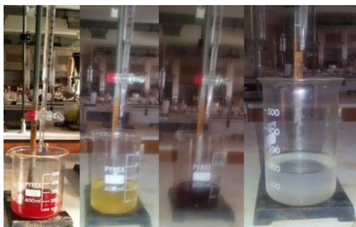
Figure : Separation process of biodiesel and glycerol
