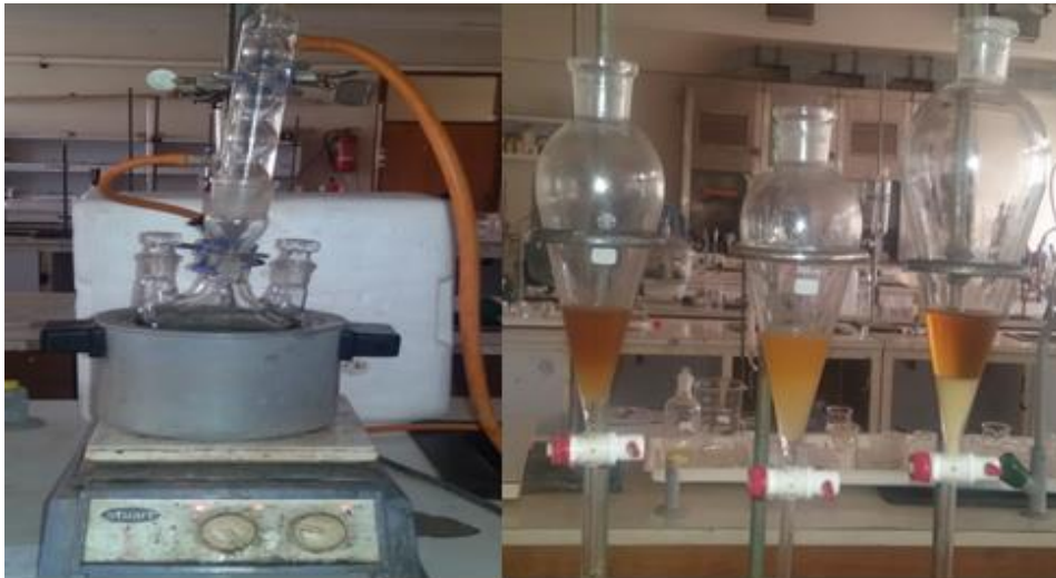
Figure 3.6: Transesterification and separation process.
