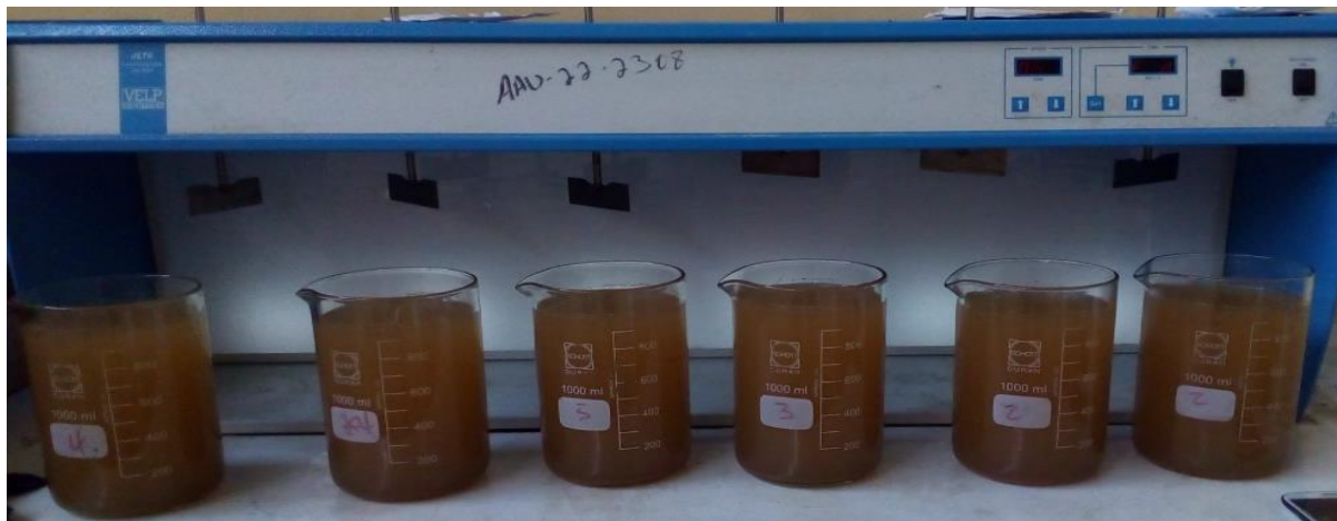
Figure 3.4 Jar test apparatus with surface water sample for coagulation flocculation treatment process.
