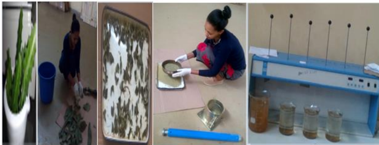
Figure 3.3 Coagulation flocculation technology for surface water treatment using cactus powder
