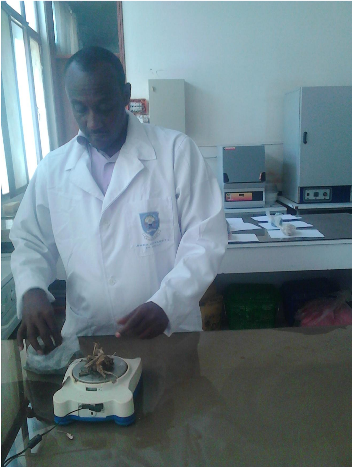
Plate 7: measuring sample waste weight for proximate analysis
