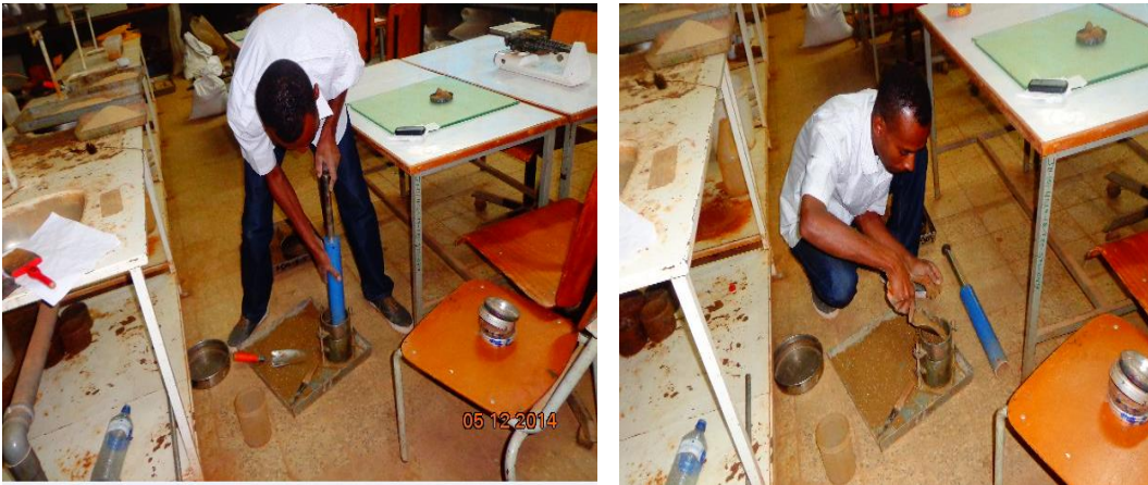
Figure 4.1. Photograph showing compaction test in laboratory
