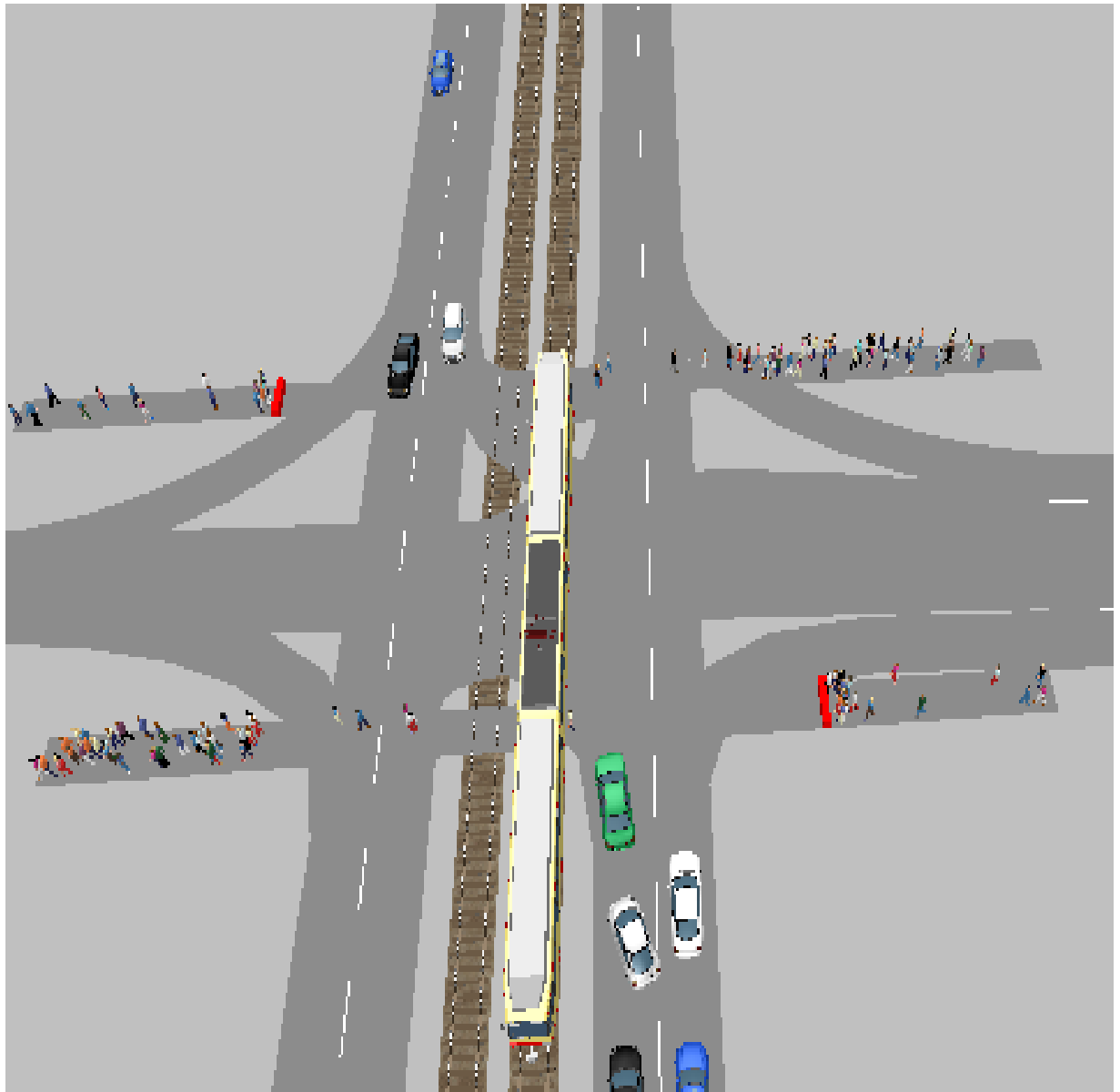
Figure: 4. 17 the condition of priority rule and geometric feature of Sebategna intersection during simulation (source: vissim simulation modeling software)
