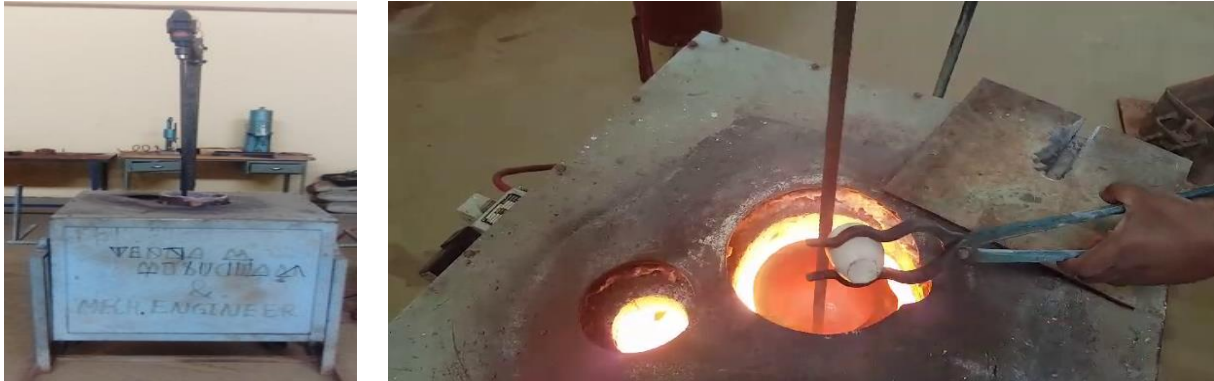
Figure B 3: Full image of stirrer machine and stirring process
