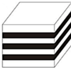
Figure 2.6: Laminated (structural) composite matrix (Przemysław et al., 2013).
