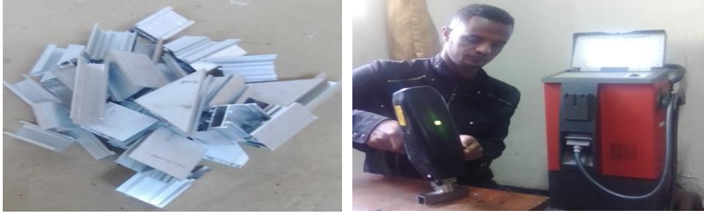
Figure B 1: Aluminum scrap and testing its composition
