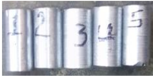
Figure 3.15: ASTM E-9 standard compression specimen
