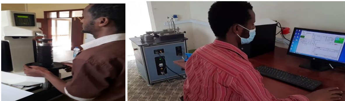
Figure B 5: Full image of Rockwell hardness test and micro pin on disc tribometer use for wear test
