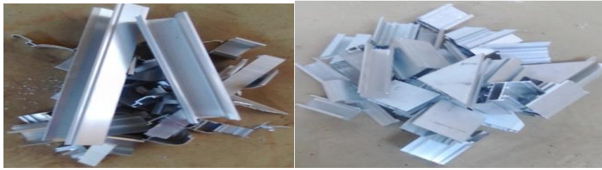
Figure 3.1: Aluminum alloy (AL-6063) scrap from life steel aluminum work
