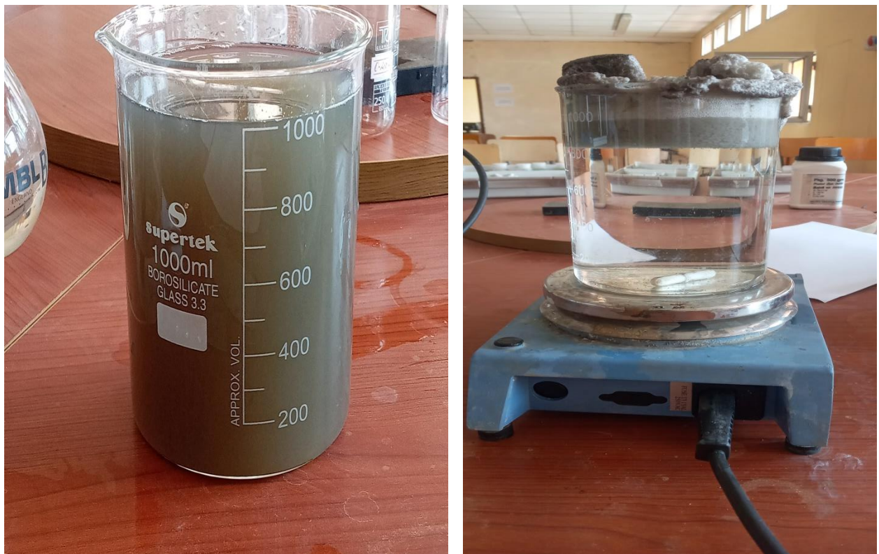
Figure E-4 before and after treatment of coffee processing of wastewater
