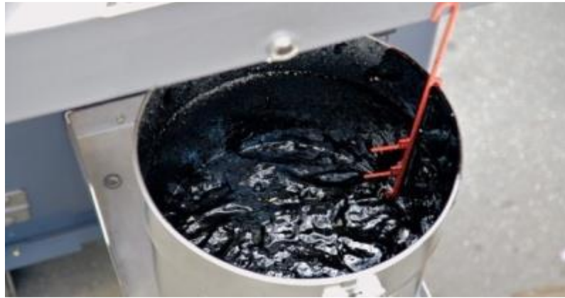
Figure .2.7.Foamed bitumen (Source: (S K Rahman*1, 2019))
