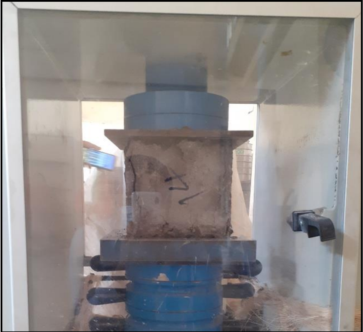
Figure 8: Pictures of cube samples in compressive test machine at JU laboratory
