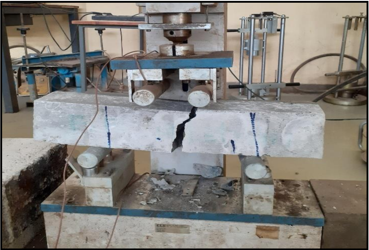
Figure 12: Pictures of beam samples in flexural strength test machine at JU Laboratory
