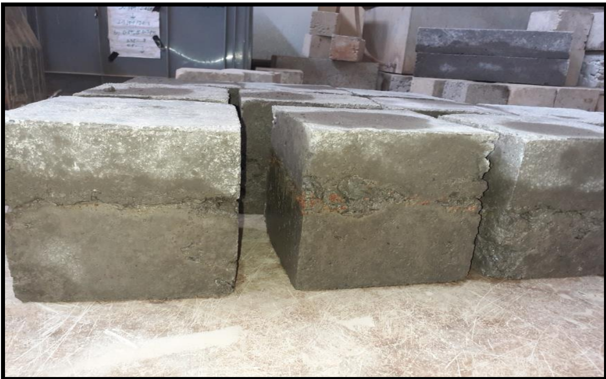
Figure 7: Pictures of cube samples with cold joint at JU laboratory
