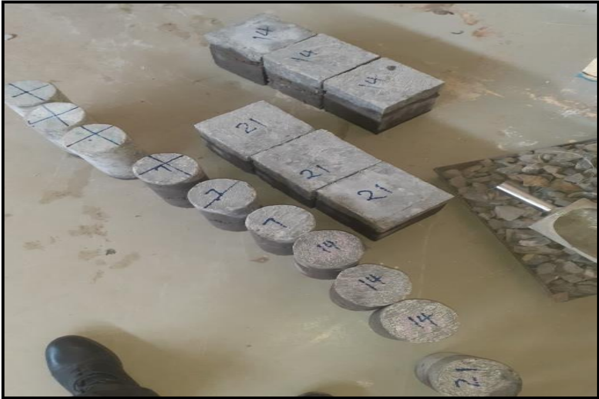
Figure 6: Pictures of samples with different cold joint formation time at JU laboratory
