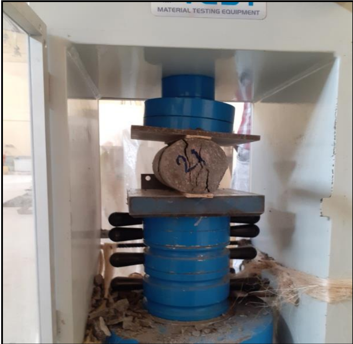
Figure 10: Pictures of cylinder samples in split tensile strength test machine at JU Laboratory
