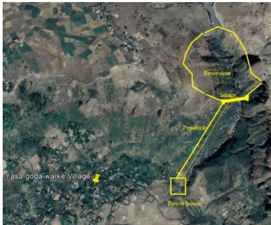
Figure 2.2: Location of suitable area for hydro power generation system on Girar River.
