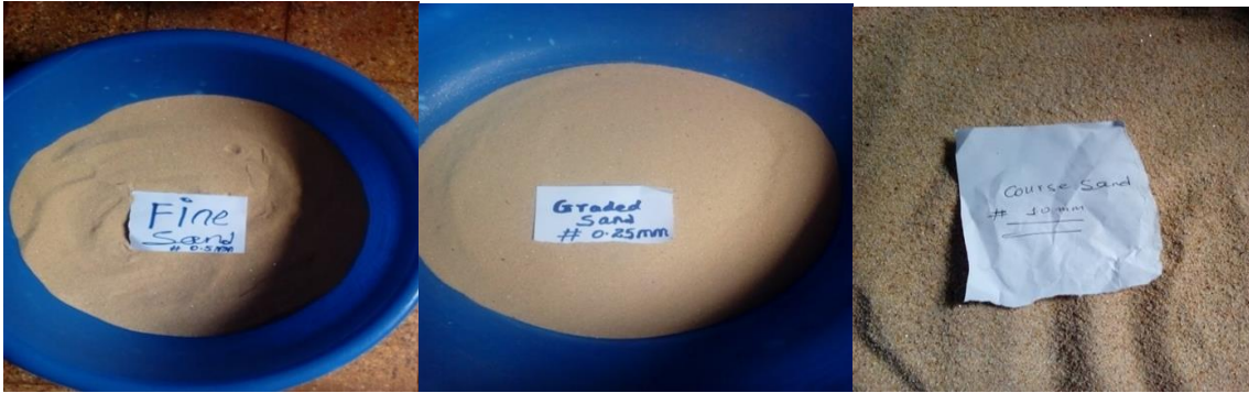
Figure (6): Types of sand after sieve analysis in the laboratory section.
