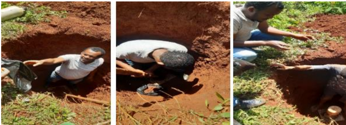
Sampling and conducting of sand cone tests
